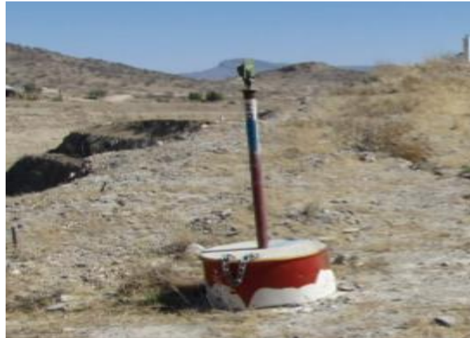
Figure 8: Recommended survey monitoring target.
