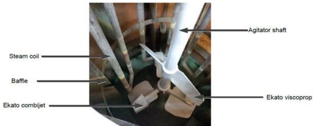
Figure 7: An illustration of the interior of the 2 m 3 test rig with EKATO Combijet impeller.
