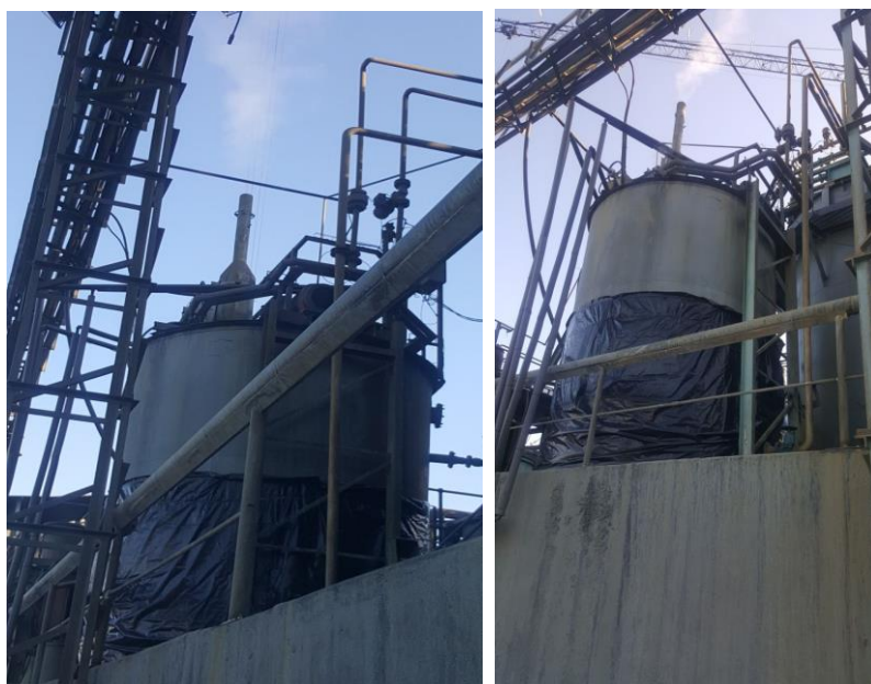
Figure 10: 21 m 3 Thermophile validation and scale-up reactor (65–68°C).
