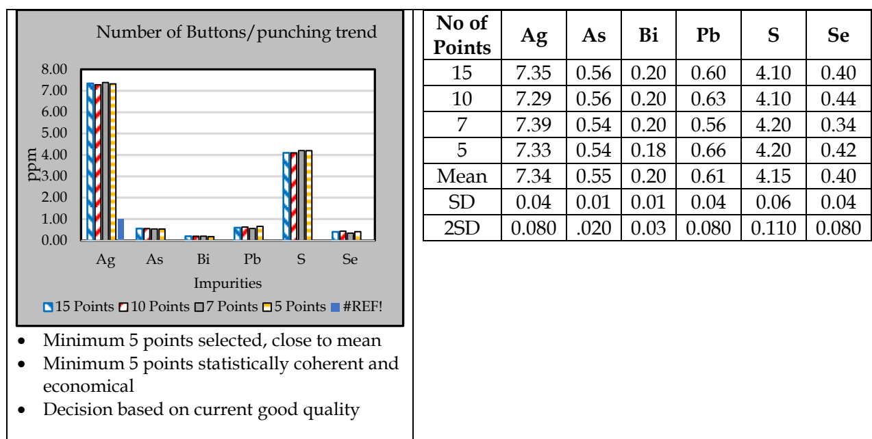
Figure 9: Established of number of points to be punched per cathode piece.
