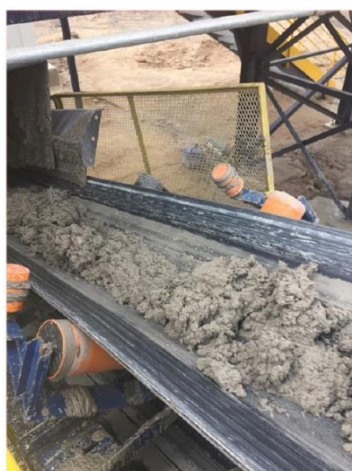
Figure 9: Centrifuge solid and liquid discharge at Lipari's Braúna Diamond Mine. (Photographs taken at Lipari diamond gold mine by Robert Klug, Flottweg SE.)
