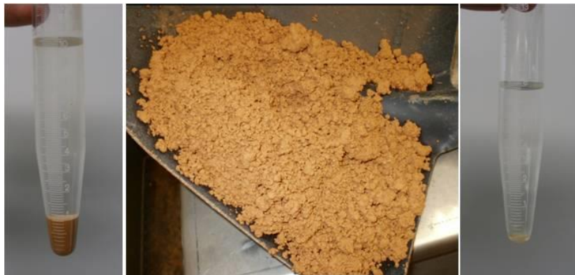
Figure 7: Photographs of feed, solid discharge and centrate from centrifuge. (Photographs taken by Robert Klug, Flottweg SE, at Sibelco sand pit mine, Italy.)
