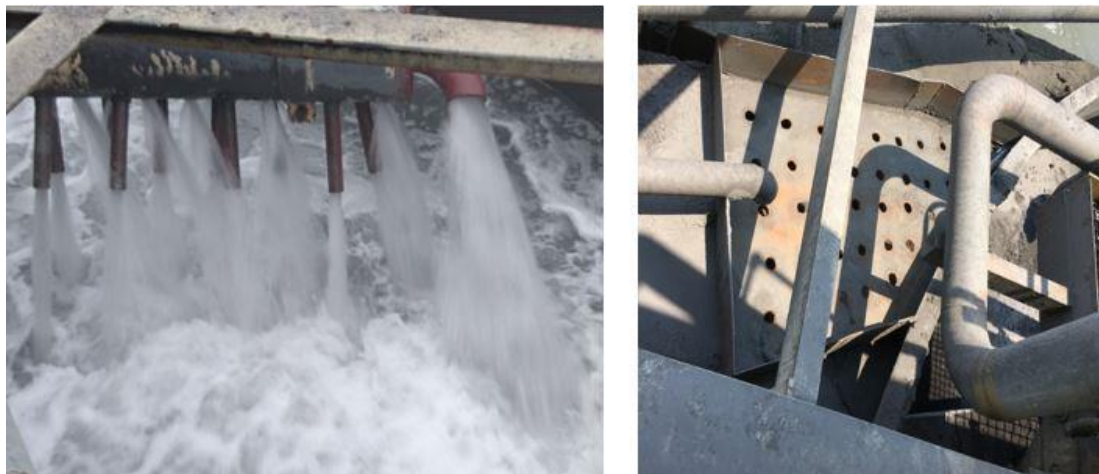
Figure 9: Improvements to flocculant distribution.
