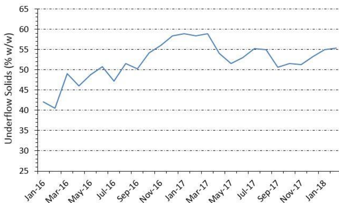
Figure 14: Monthly Underflow density trends 2016-2018 (SCADA data).
