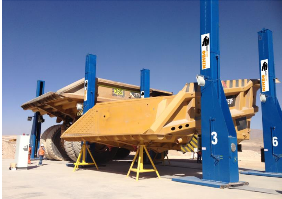
Figure 7. Back view of the KIMBO system – Truck prepared to remove the old body and in the second work zone, a new one on support stands.
