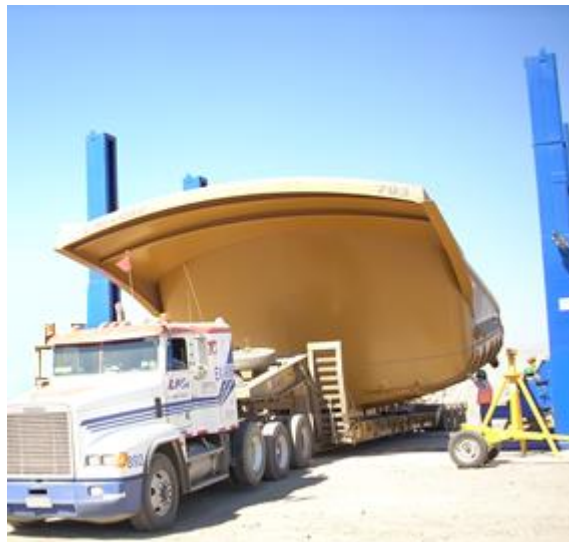
Figure 6. Front view one work zone of the KIMBO system – Low boy truck bringing a new dump body.
