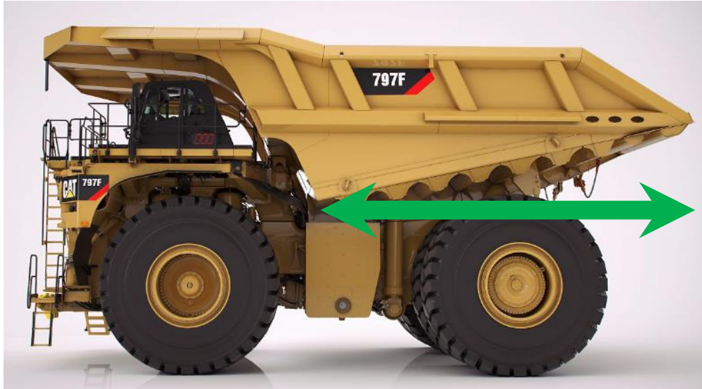
Figure 8. The green arrows indicate the “KIMBO dimension” required to assess whether the system can handle a particular dump body.
