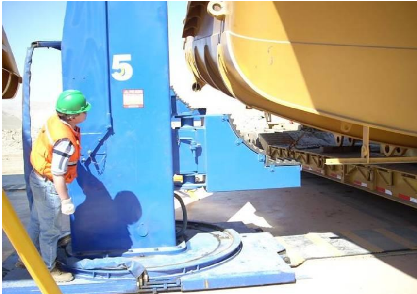
Figure 5. Central, rotating column of the KIMBO system.
