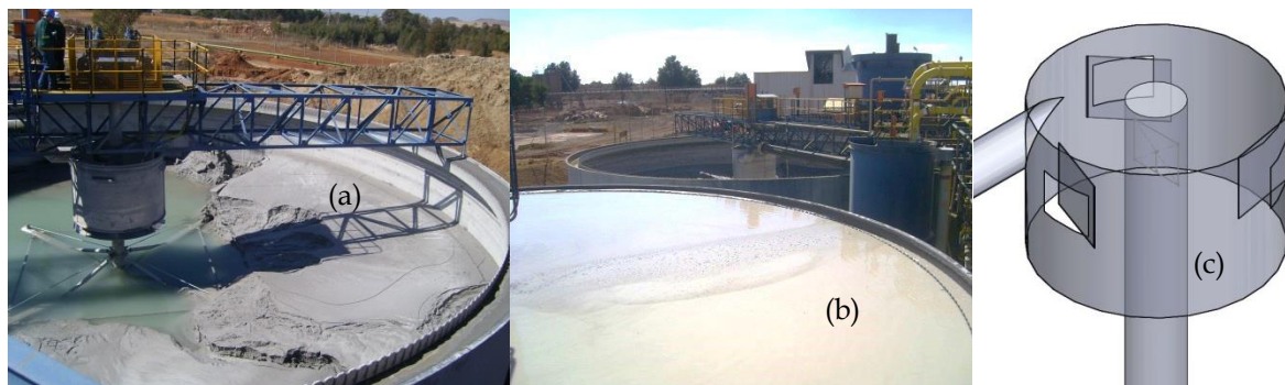
Figure 3. (a) Stalled and drained thickener with original open feedwell (with deflector plate). (b) Sliming thickener (with dilution slot modification), and (c) computer-aided design (CAD) drawing of the modified feedwell (with enlarged slots and added deflection baffles, deflector plate not shown).
