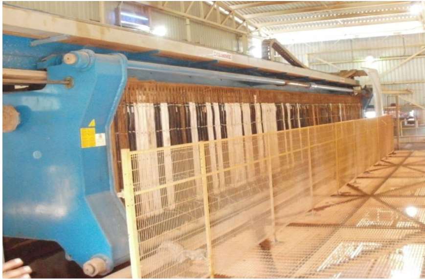
Figure 6. Chamber filter press. (Photograph taken by Robert Klug, Flottweg SE, at La Sopresa Minera Mine, Mexico.)
