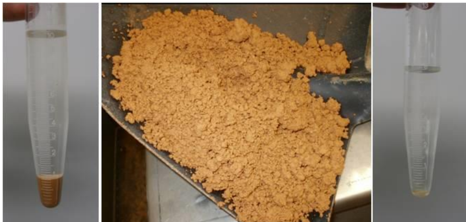
Figure 12. Photographs of feed, solid discharge and centrate from centrifuge. (Photographs taken by Robert Klug, Flottweg SE, at Sibelco sand pit mine, Italy.)
