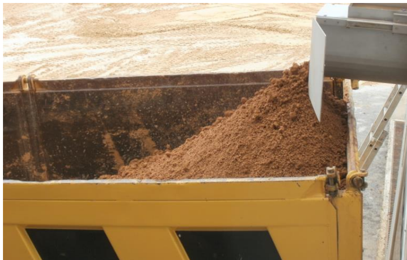
Figure 10. Continuous discharge of solids after centrifugation. (Photograph taken by Robert Klug, Flottweg SE, at Sibelco sand pit mine, Italy.)
