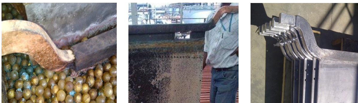
Figure 7. Progressive evolution in hanger bar design.
