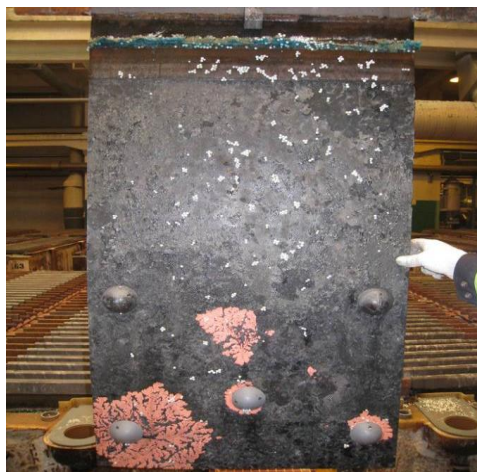
Figure 10. Copper plating on lead anode (With permission to reproduce from Nikkelwerk, 1/26/2014).
