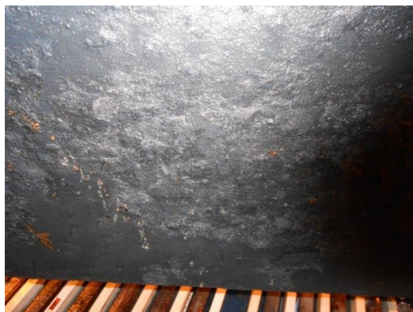
Figure 3. Hard, dense, adherent \alpha -PbO 2 (brownish colour).
