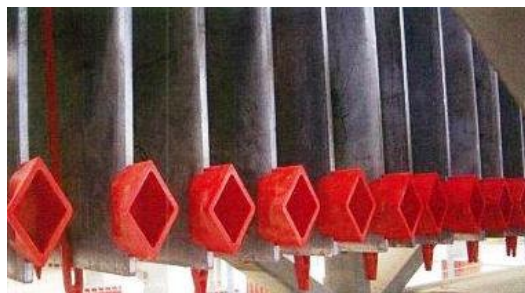
Figure 1. Typical anode spacers in common use in EW plants.
