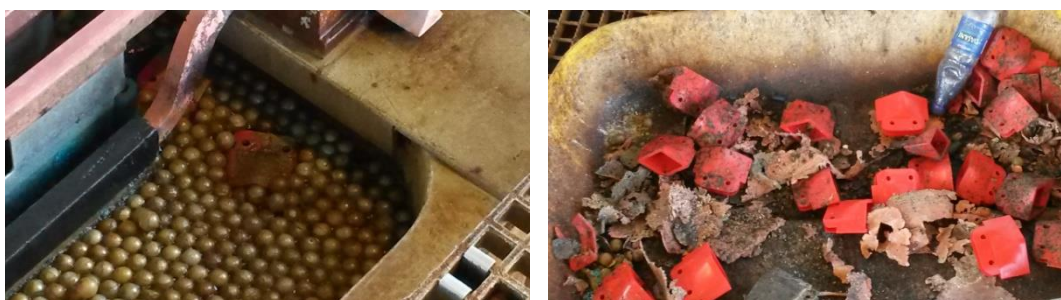
Figure 2. Dislodged and damaged anode spacers.
