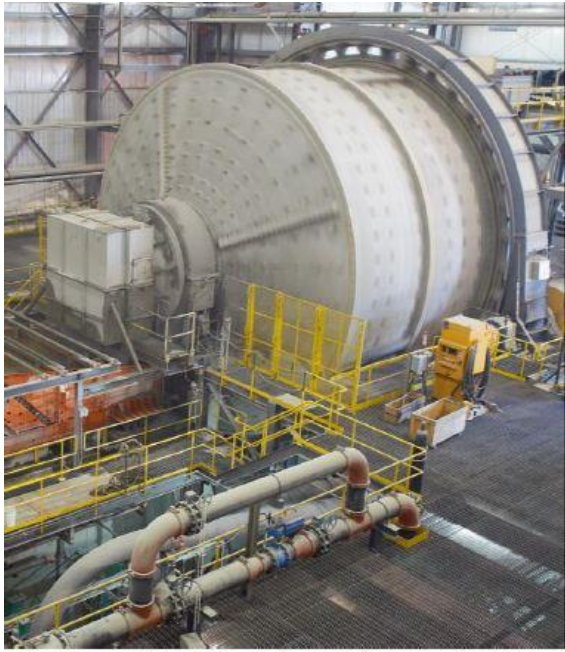
Figure 3. 10.4 m x 6.1 m F/F SAG mill.
