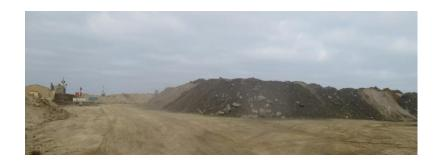
Looking at ToC the bottleneck was the ability of L&H to achieve required plant feed rates. This justified the creation of a buffer stockpile ahead of the tipping bin.
