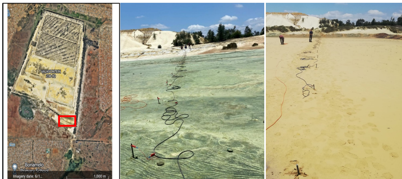
Figure 1. Electrical resistivity tomography tests on two terraces of the TSF (left) green terrace and (right) yellow terrace.
