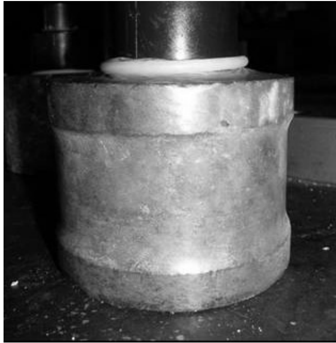
Figure 10 Specially prepared doorstopper sample
