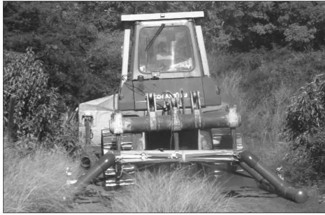
Figure 1—Towed 25 MHz GPR system surveying at RBM
