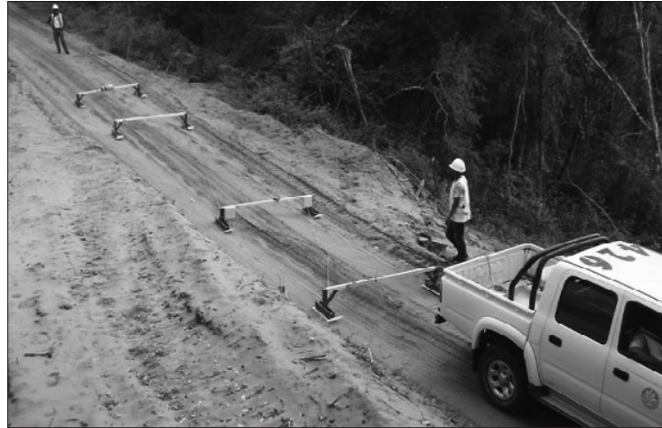
Figure 3—Prototype custom ultra-deep GPR system being trialed on RBM sands
