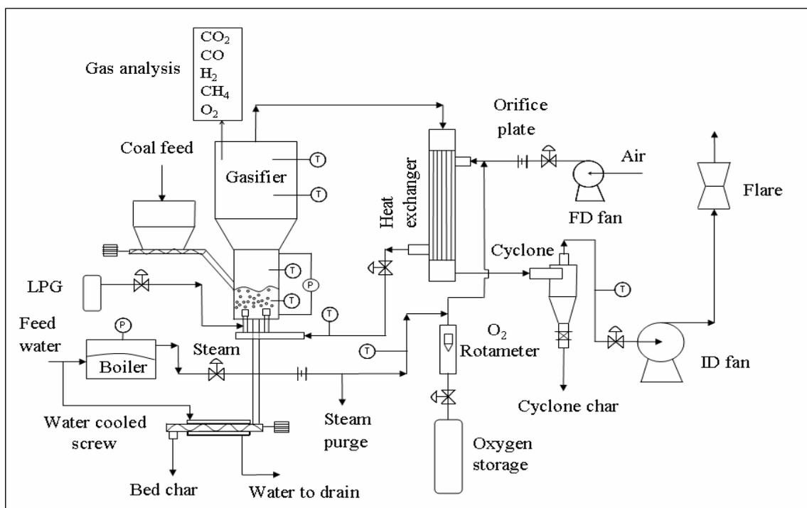
Figure 1. Pilot-scale fluidized-bed gasification plant
