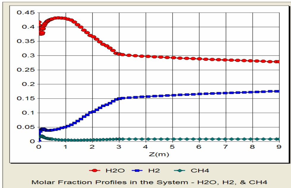
Figure 8. Mole fractions of H<sub>2</sub>O, H<sub>2</sub> and CH<sub>4</sub> as a function of gasifier height
