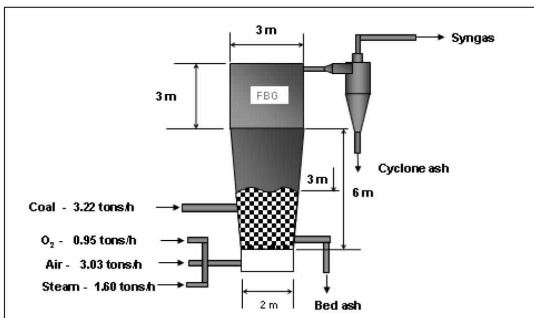
Figure 5. 15-MW fluidized-bed coal gasifier
