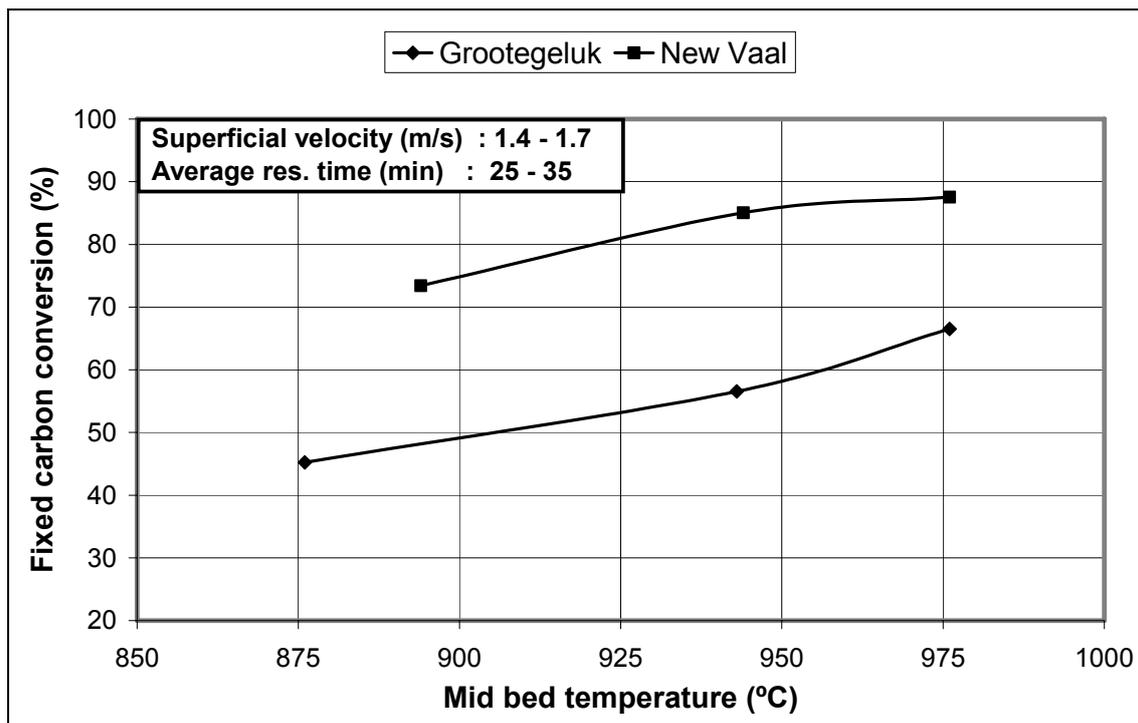
Figure 2. Fixed-carbon conversion as a function of temperature
