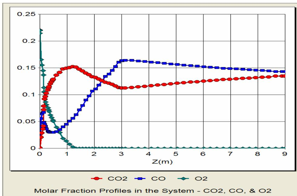
Figure 7. Mole fractions of CO<sub>2</sub>, CO, O<sub>2</sub> as a function of gasifier height
