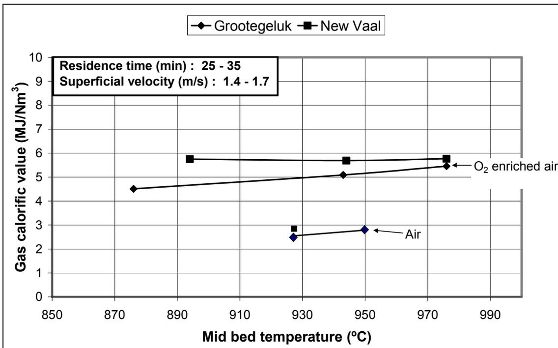
Figure 4. Gas calorific value as a function of temperature
