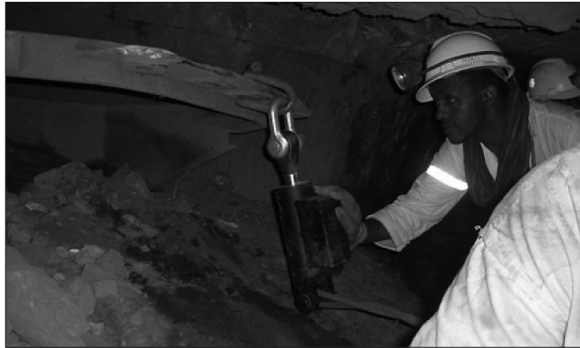
Figure 5. Attaching the device to the scoop
