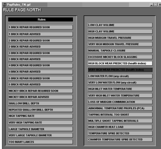
Figure 8. Rule page display showing active rules triggering a yellow or red warning
