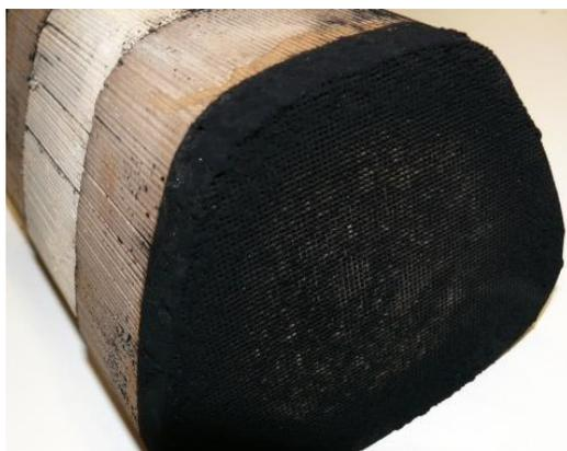
**Figure 5-Carbon-contaminated monolith**
