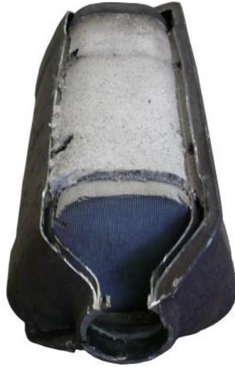
**Figure 3-Spent catalytic converter**
