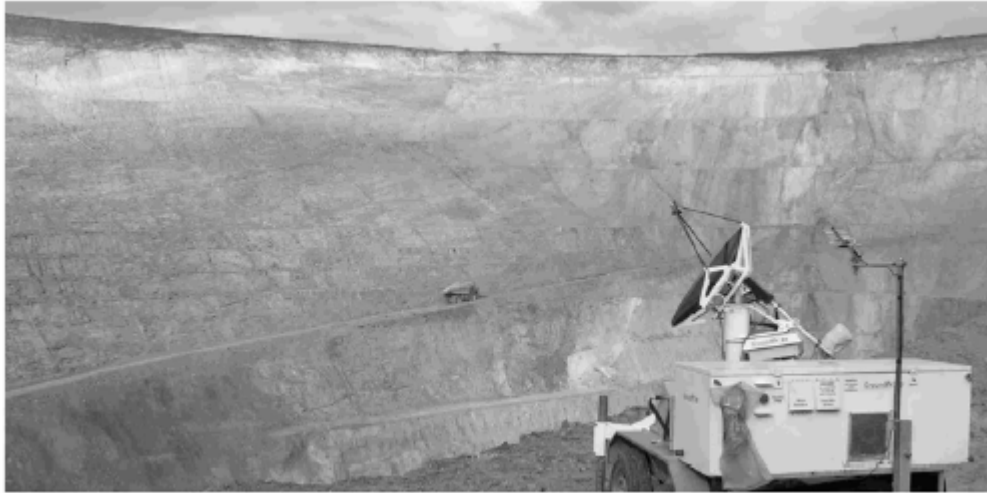
Figure 5 Groundprobe's Slope Stability Radar, monitoring the south east wall at Harmony.
