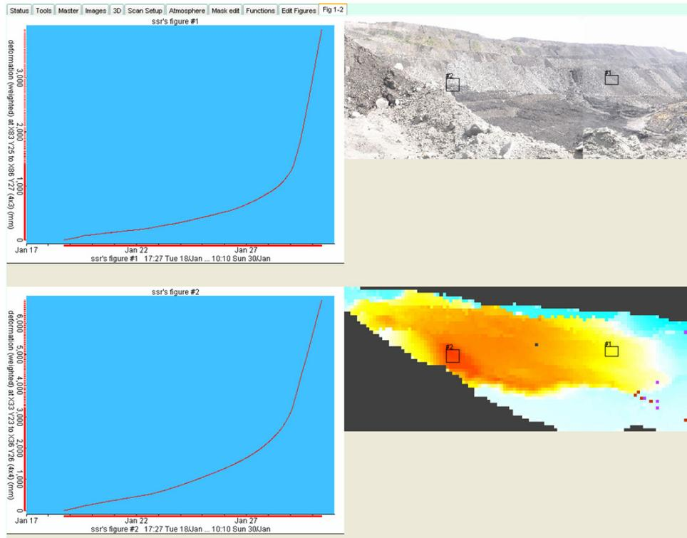
Figure 1: SSR Visual of the Mt Owen Wall Failure (with Selected Displacement Plots)
