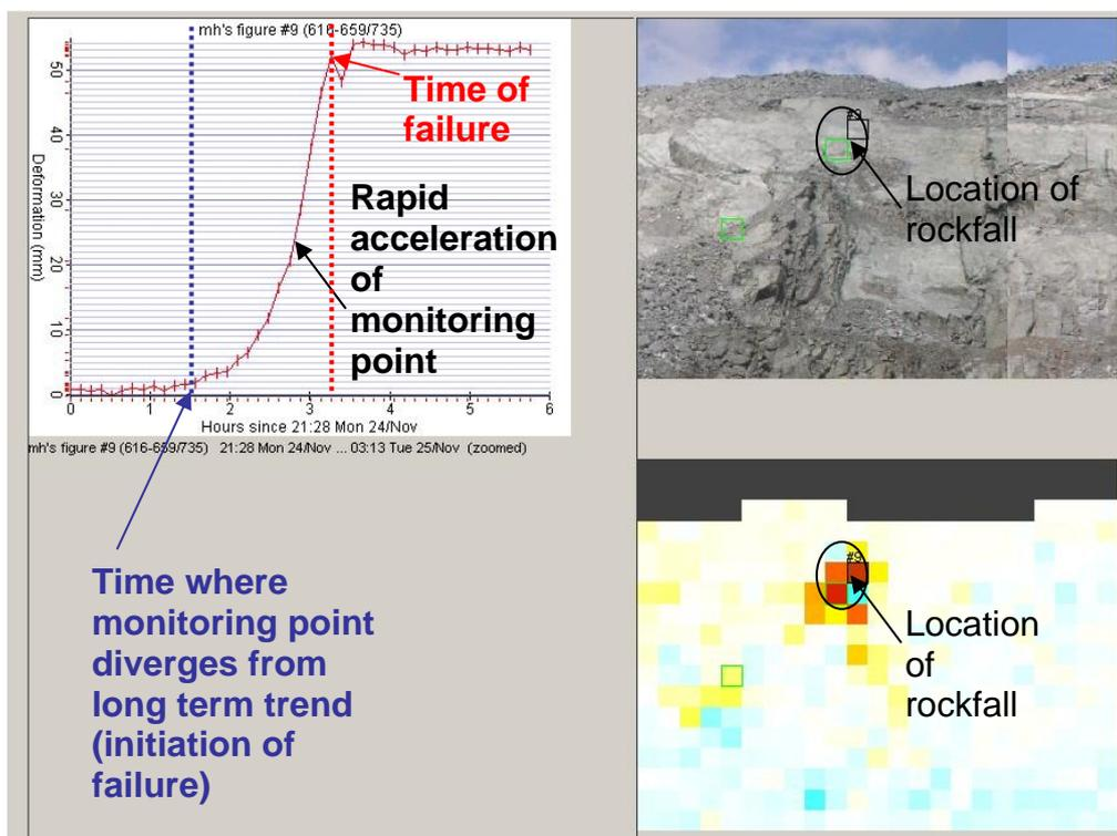
Figure 3: SSR visual of the Rock Fall (with Selected Displacement Plot)
