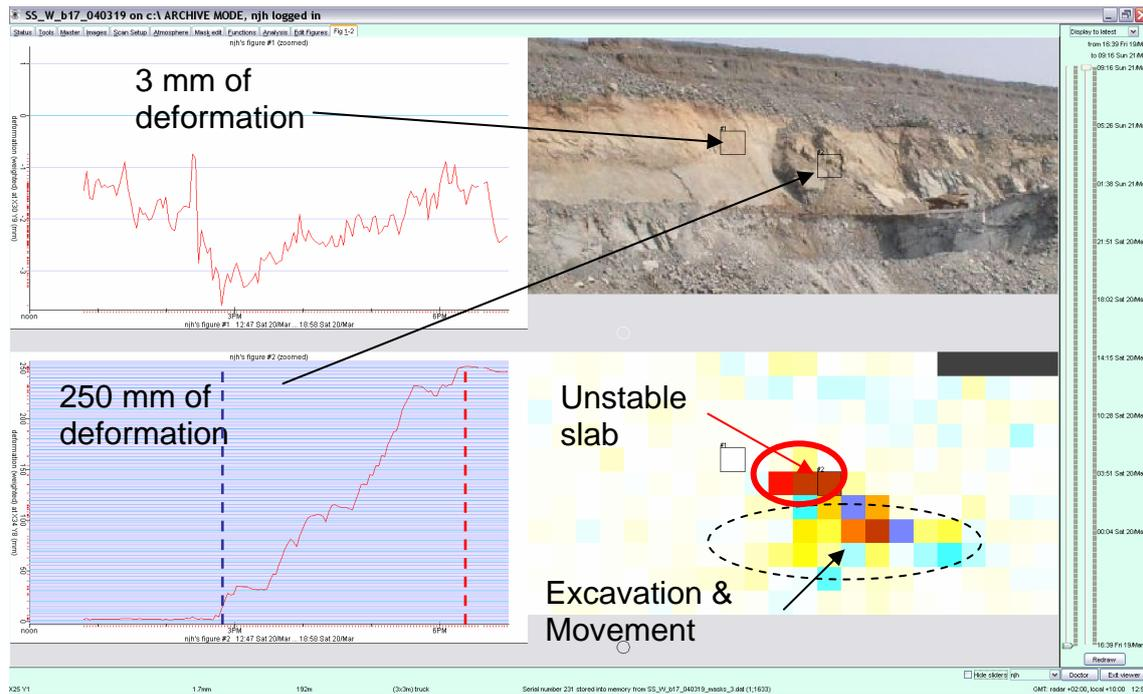
Figure 5: SSR Visual of the Rock Slab Failure Caused by Undermining the Toe
