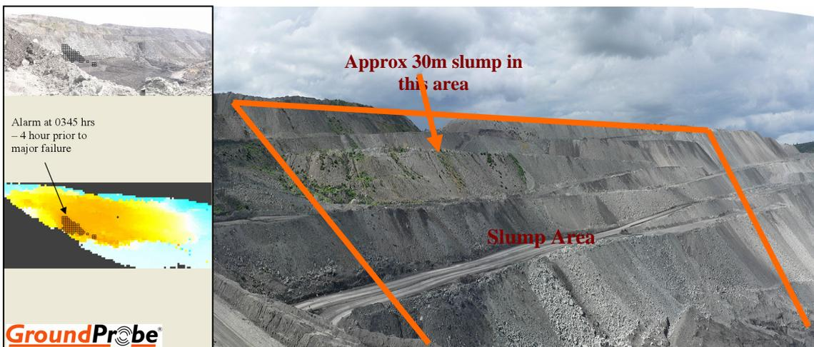
Figure 2: Visual of Alarm Trigger and Failure Surface
