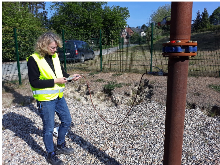
Figure 6. Sampling of mine gas at a Protego hood to sample mine gas and determine the gas composition and concentration (Photo: B. Teichert, THGA).
