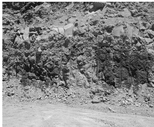
Figure 12: Level 830-815, NPK Kimberlite Rock (Splitex 25 mm Diameter)
