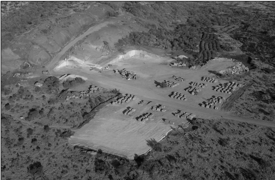
Figure 5 The W2 quarry at Wonderkop showing orderly quarry development, stockpiling of topsoil removed from areas required for infrastructure, and removal of topsoil ahead of waste dumping.
