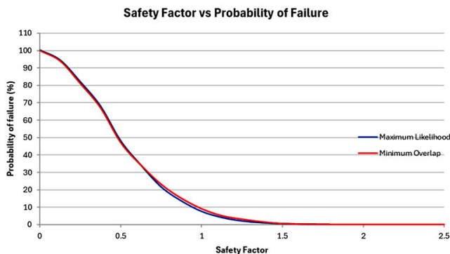
Figure 5—Factor of safety vs probability of pillar failure (Van der Merwe, Mathey, 2013b)
