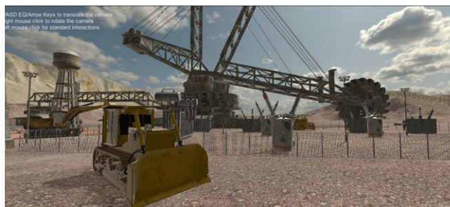
Figure 3—Dozer and bucket wheel excavator
