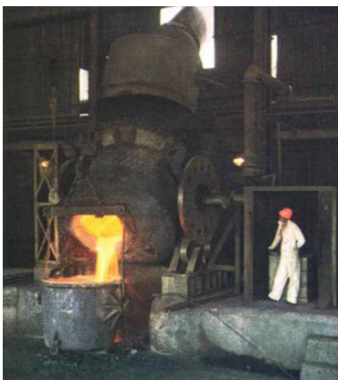
Figure 2—(left) The processing operations at Klipfontein with the smelter shown in the foreground next to the stack; (right) Pouring blown matte from one of the converters (after Johnson Matthey, 1969)
