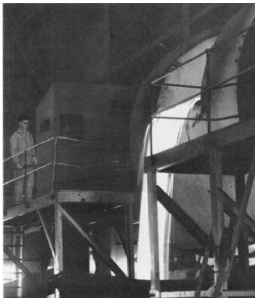
Figure 13—(left) Skimming slag from the Peirce Smith converter at Waterval (after Johnson Matthey, 1970); (right) 3D model image of the CP TSL (after Hoosen et al., 2018)
