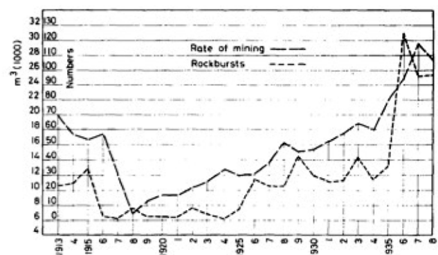
Figure 1—Relationship between rockburst incidence and mined volume for the Brezove Hoty mine district in Czechoslovakia (Cook, 1976)
