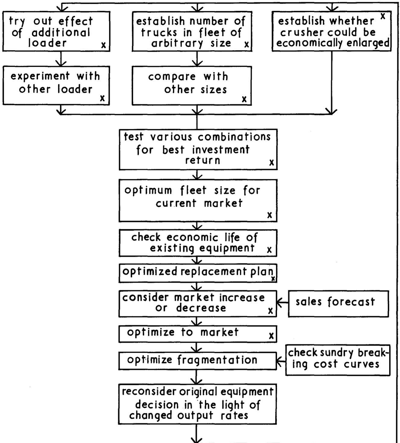
Fig. 8—Logic diagram of stages in equipment selection
