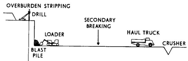
Fig. 2—The quarry process
