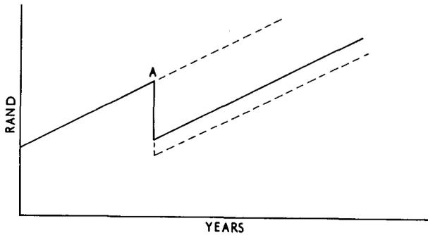
Fig. 4—Level of operating costs if a machine is replaced
