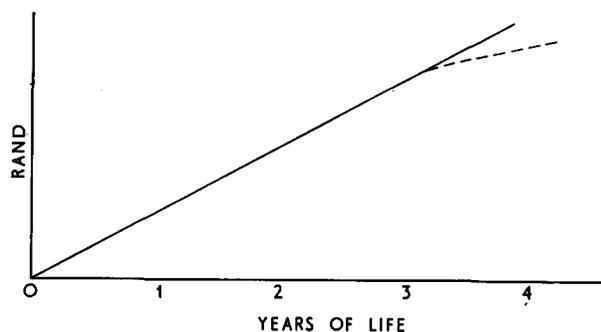
Fig. 3—Increase in cost of operation of a machine with age
