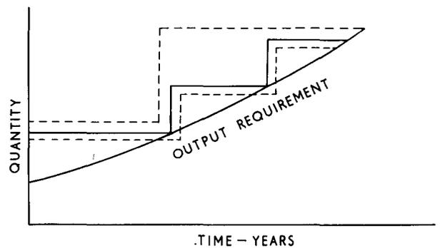
Fig. 5—Diagrammatic presentation of plant capacities required for increasing output
