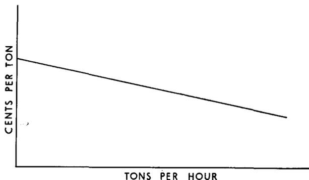
Fig. 7—Decreasing loader costs with increasing loading rate
