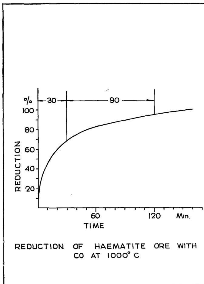
Fig. 1—Reduction of Haematite Ore with Co at 1000°C
