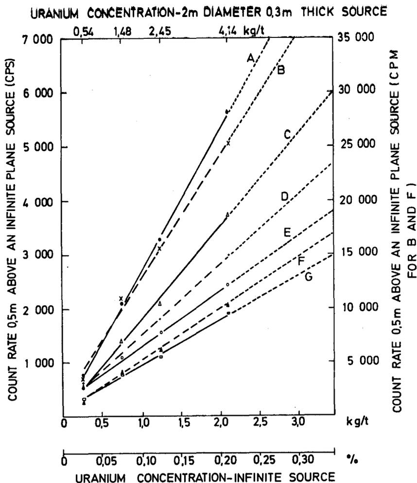
Fig. 1—Calibration curves obtained for different gamma survey meters
