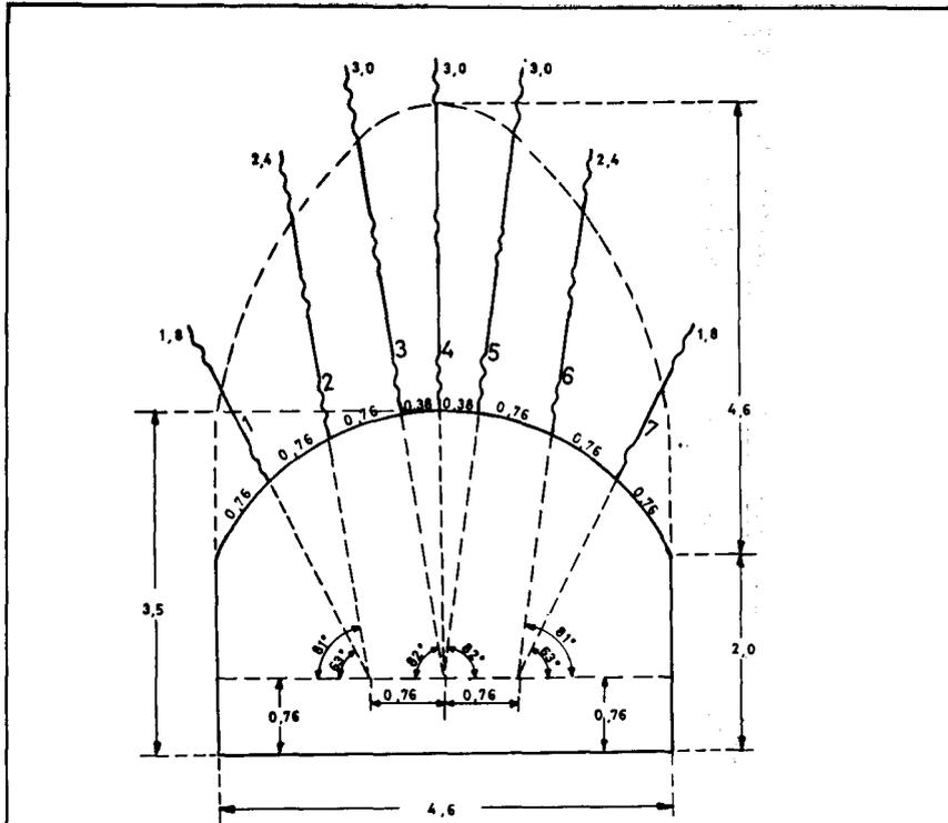
Roof bolt pattern for 4,6 x 3,5m. drives in weak rock formation.
