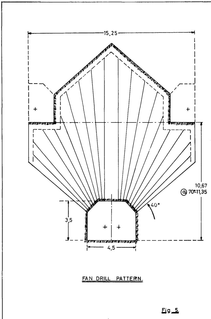
of the drift. Toe spacing will then be 0,9 m.
