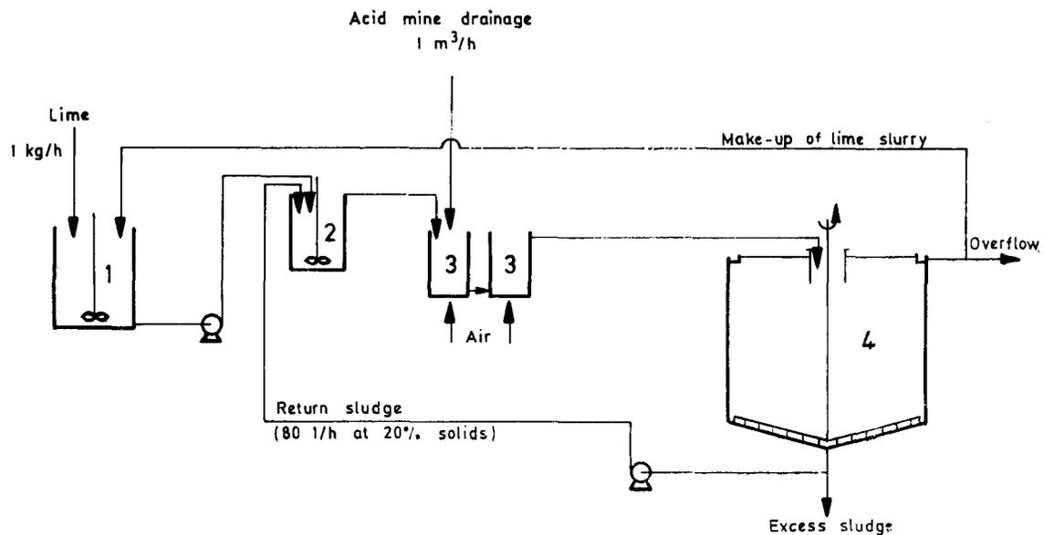
**Fig. 3—Flow diagram for the pilot plant**
