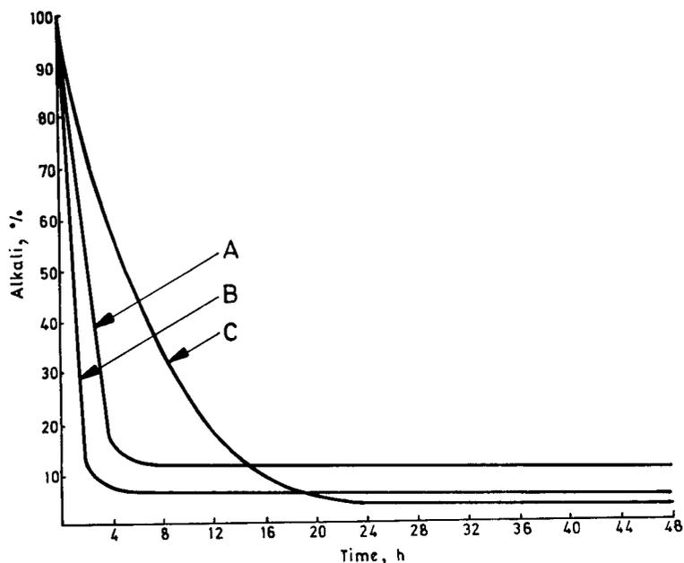
**Fig. 1—Settling rate of precipitate from Kromdraai neutralized water**
