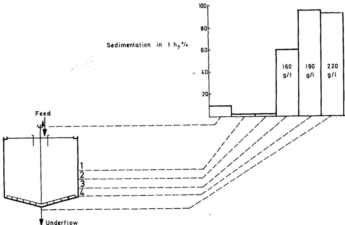
Fig. 4—Density profile of the sludge in the thickener
