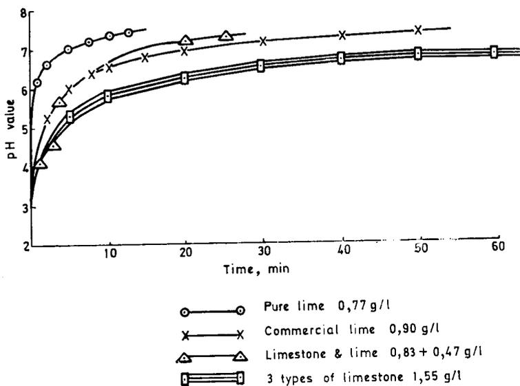
**Fig. 2—Neutralization of Kromdraai acid drainage with different types of lime and limestone**
