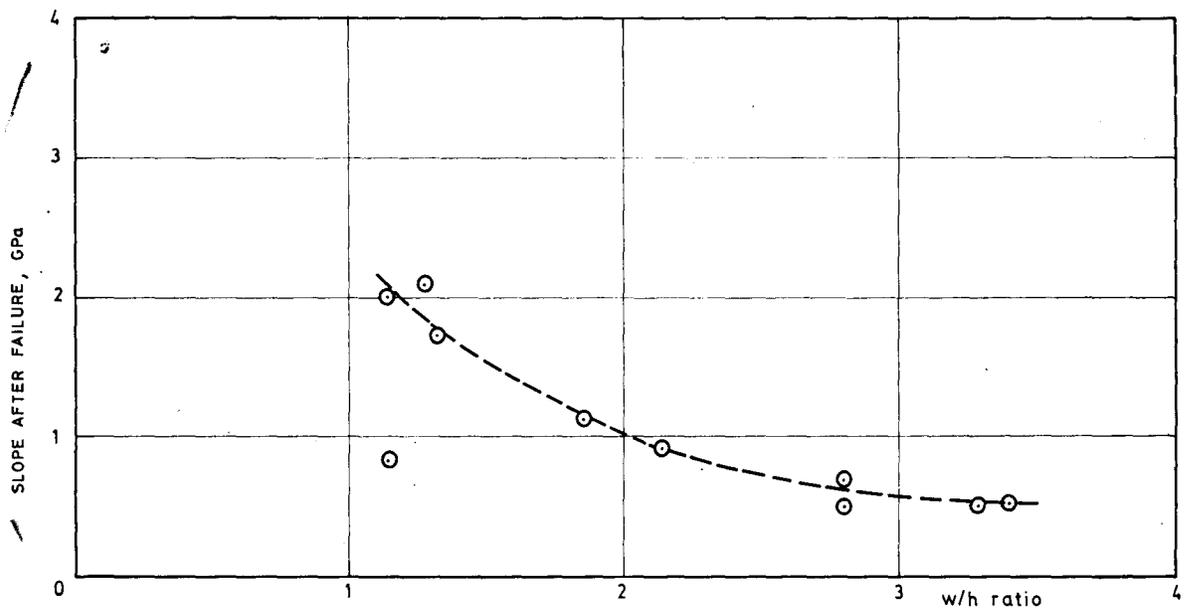
Fig. 10—Influence of  $w/h$  ratio on the slope of the stress strain curve after failure
