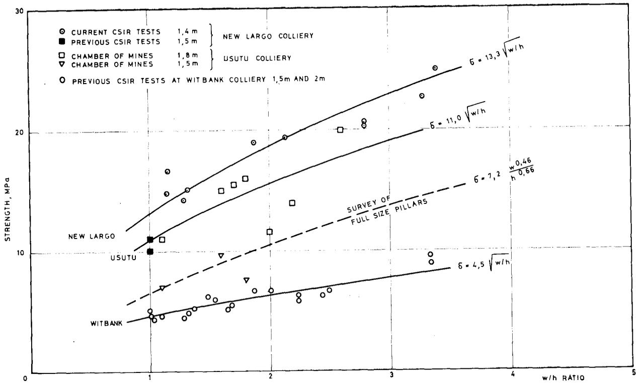
Fig. 7—Comparison of current strength data with those of previous tests
