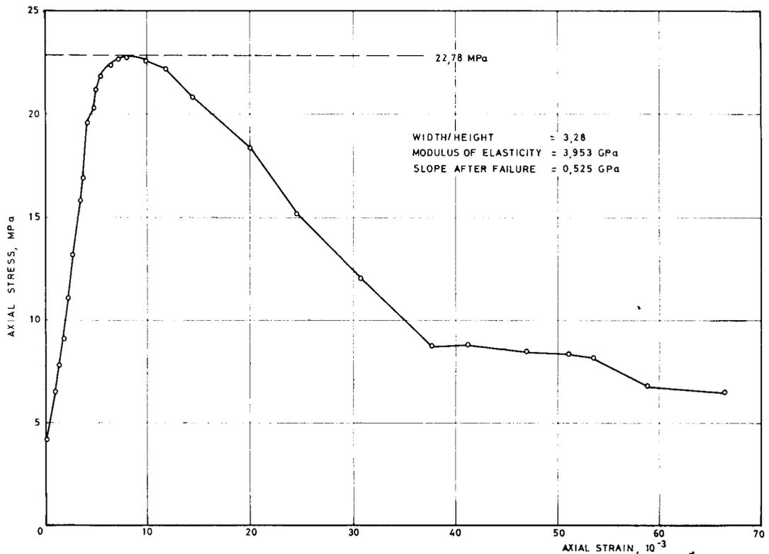
Fig. 6—Complete stress-strain curve obtained for specimen No. 9
