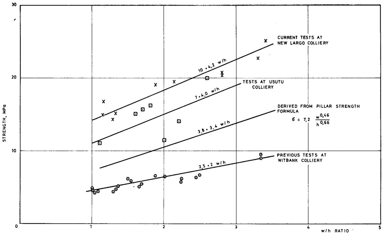
Fig. 8—Representation of strength data by a straight line
