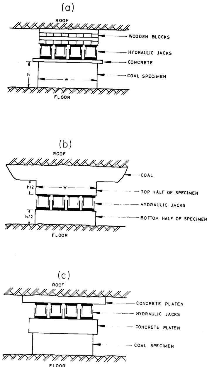
Fig. 3 (a) Stress-controlled loading of coal specimens (after Bieniawski<sup>2</sup>)
