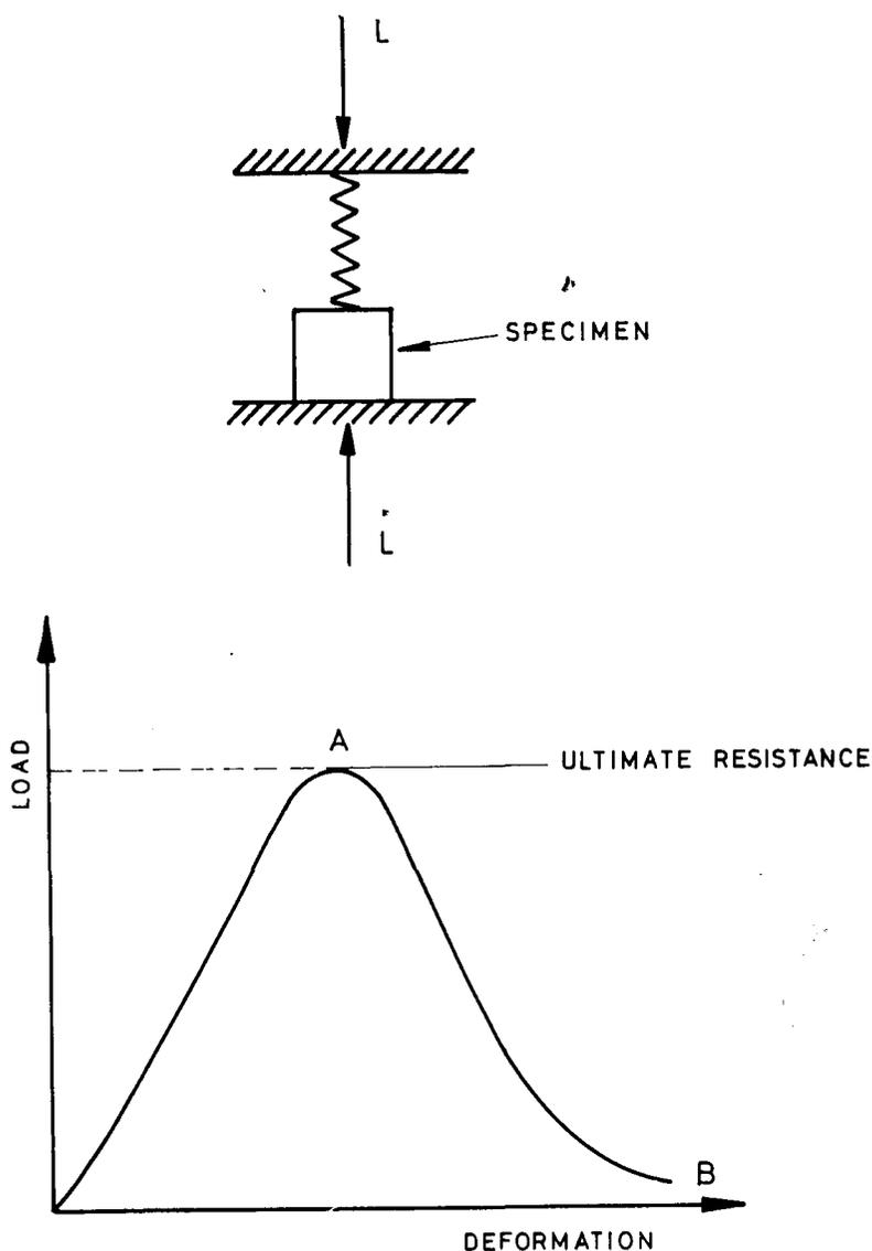
Fig. 1—Diagrammatic representation of specimen deformation under compression
