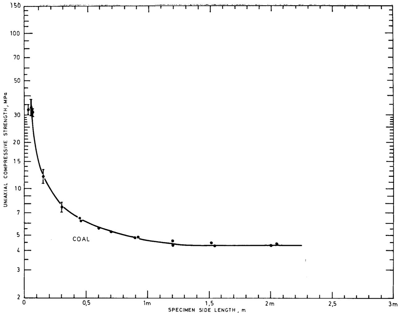
Fig. 2—The phenomenon of the strength approaching asymptotically a constant value (after Bieniawski<sup>3</sup>)
