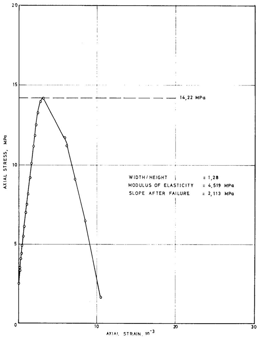
Fig. 5—Complete stress-strain curve obtained for specimen No. 3
