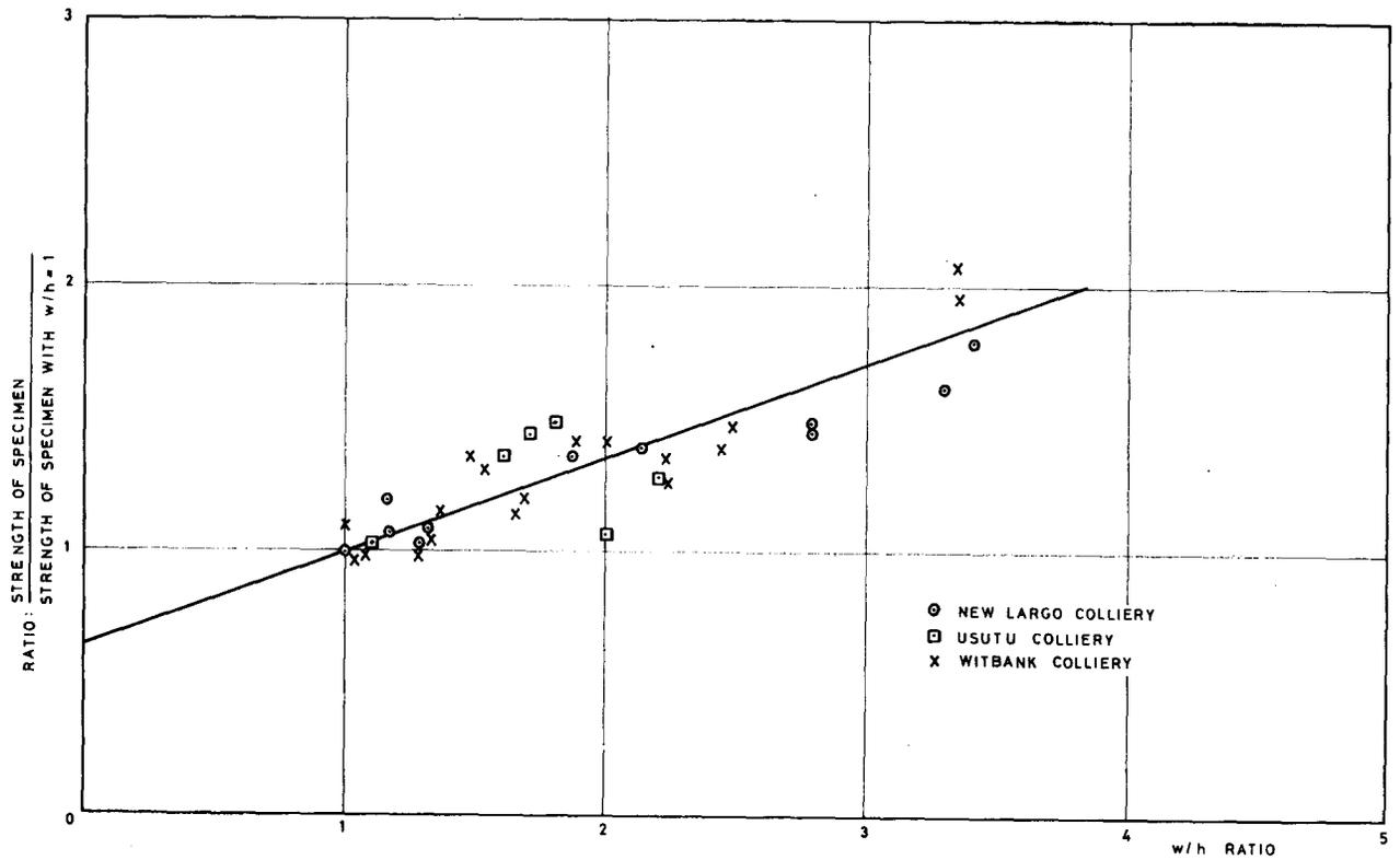
Fig. 9—Representation of strength data in dimensionless form
