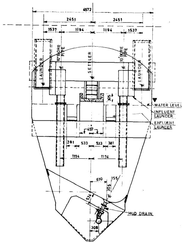
Fig. 4—Settler of Harvie Watt shaft, 25 minus 60 level at Libanon
