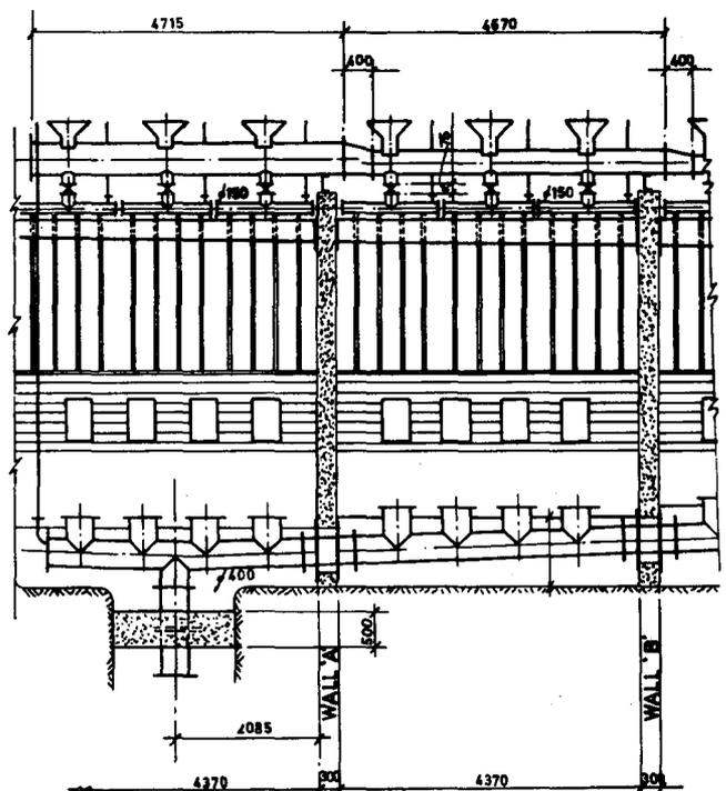
Fig. 19—Arrangement of mud settlers, 24 level No. 1 shaft, Venterspost
