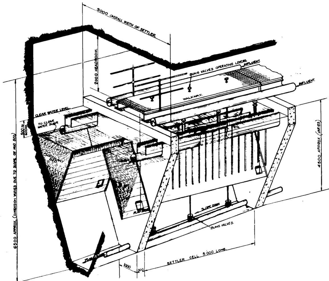
Fig. 2—Alternative arrangement to that shown in Fig. 1; this formed the basis for the Gold Fields standard settler
