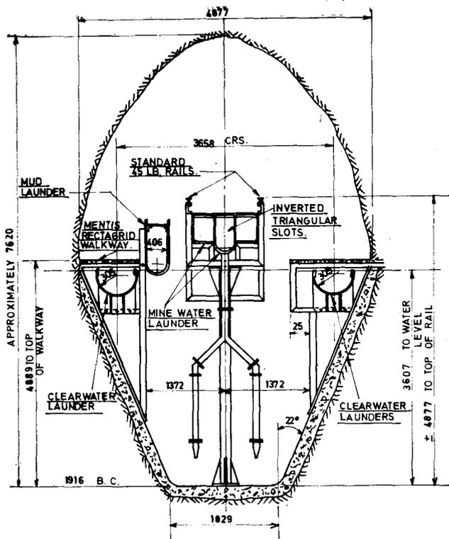
Fig. 6—No. 1 settler of No. 1 main shaft, 23 minus 60 level at Kloof
