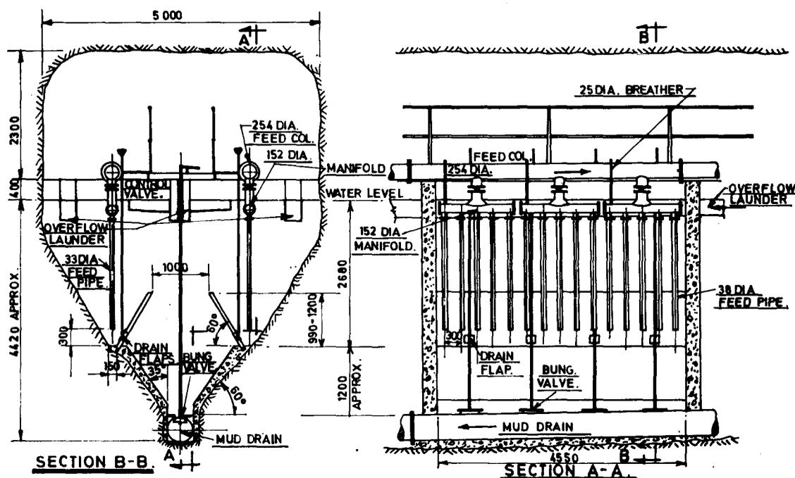
Fig. 10—Recommended layout of settler cell for an influent flow of 60,6 l/s
