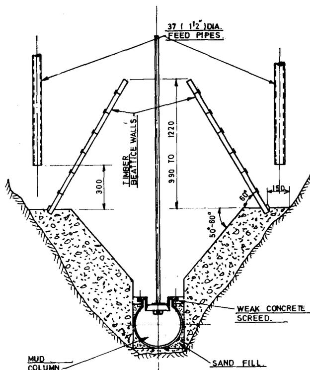
Fig. 15—Recommended arrangement for the mud outlet
