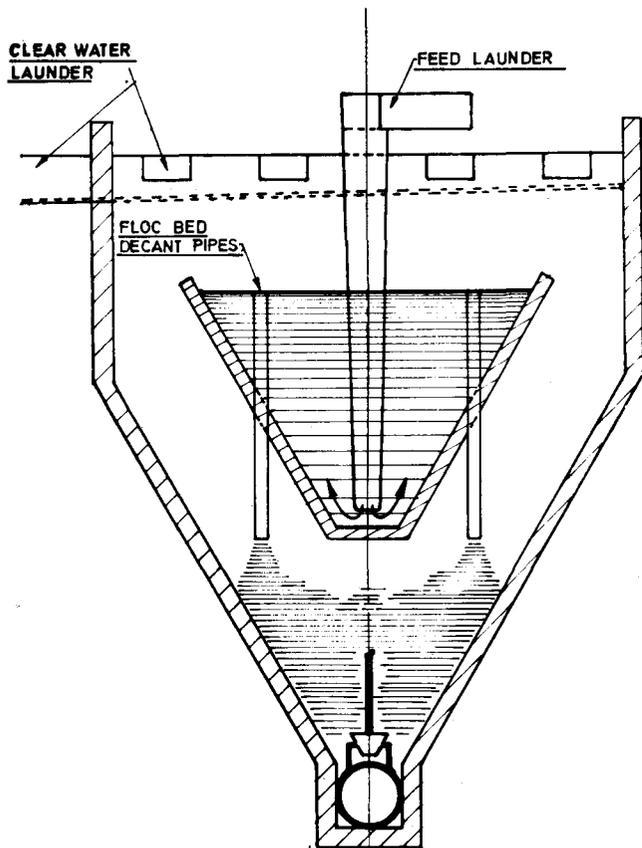
Fig. 1—General arrangement of a settler based on the findings of the Gold Fields investigation<sup>1</sup>
