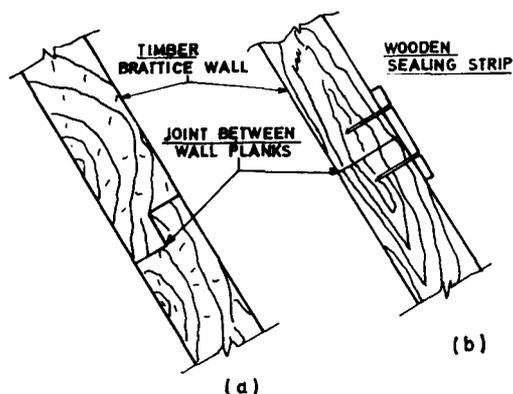
Fig. 13—Recommended joint between the planks forming the brattice walls
