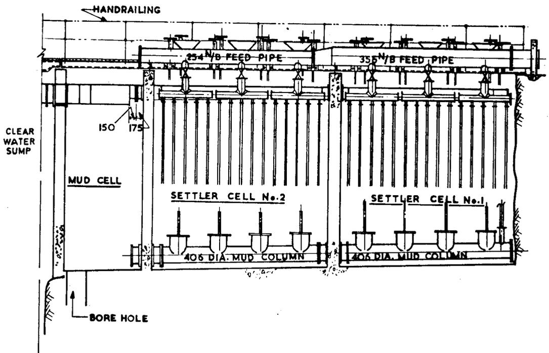
Fig. 16—Elevation showing the settlers of No. 2 shaft at East Driefontein
