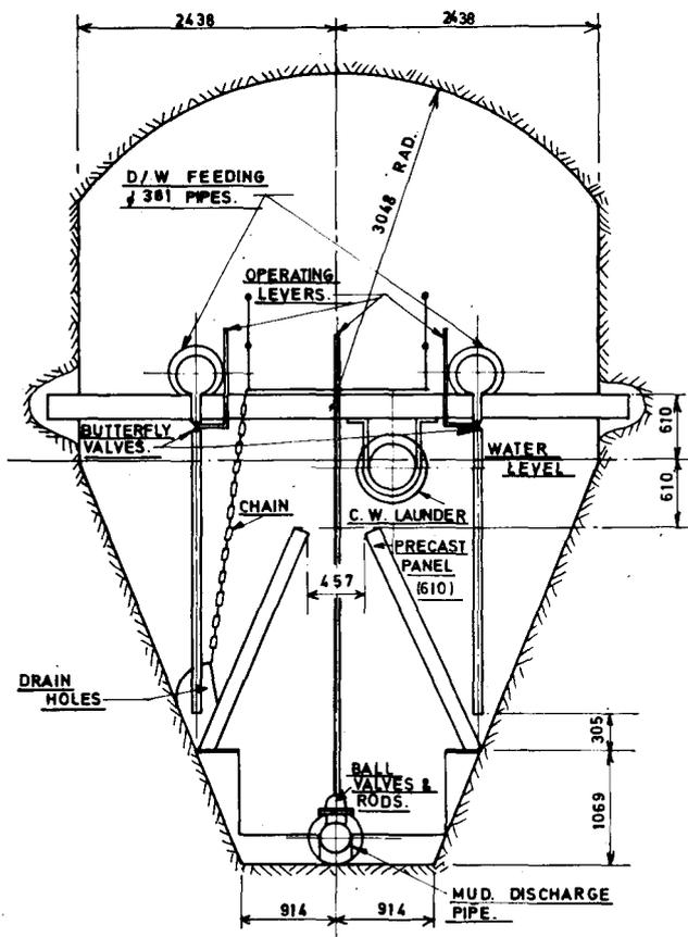
Fig. 7—No. 2 settler of No. 1 main shaft, 23 minus 60 level at Kloof
