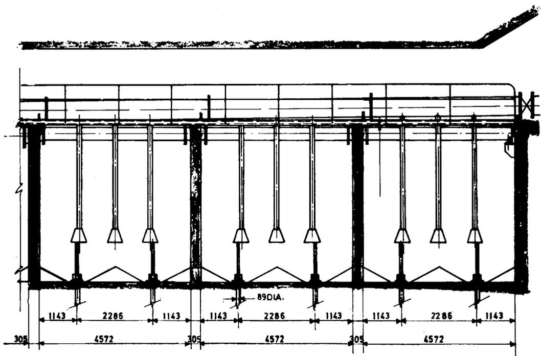
Fig. 5—Settler of No. 2B tertiary shaft, 26 level at Venterspost
