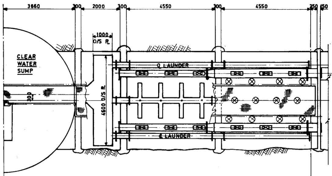
Fig. 17—Settlers of No. 2 shaft at East Driefontein
