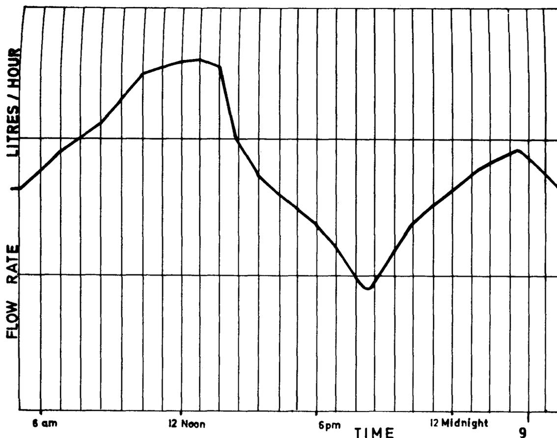
Fig. 9—Typical curve showing water flow rate for 24 hours
