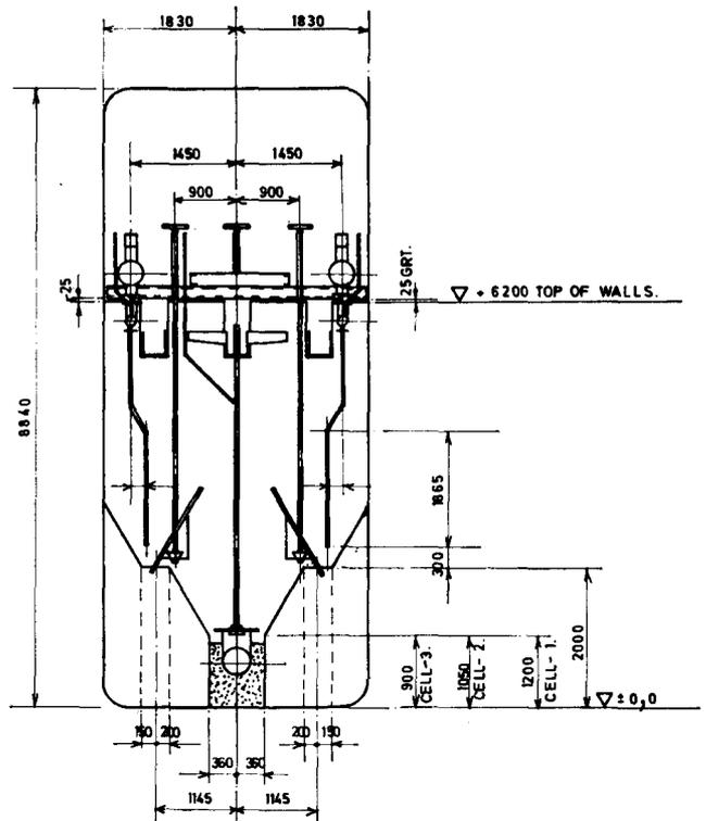
Fig. 18—Arrangement of mud settlers, 24 level No. 1 shaft, Venterspost
