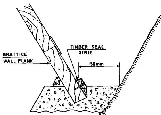
Fig. 14—Detailed view of the bottom of the brattice wall
