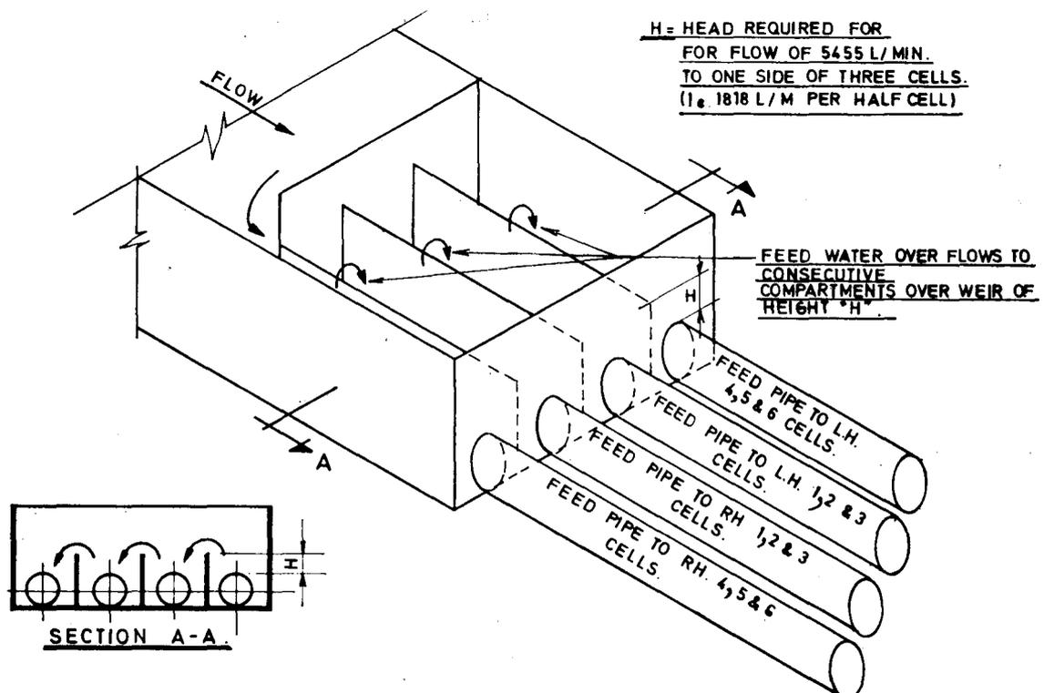
Fig. 11—Feed launder for constant feed to the cell
