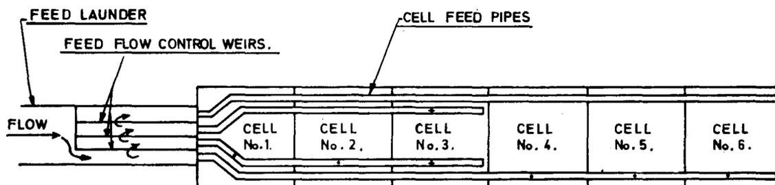
Fig. 12—Plan of feed launder and pipes for a six-cell settler, each pipe being designed to accommodate the feed to three half-cells
