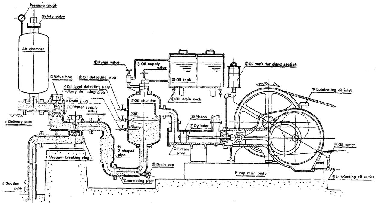
Fig. 1—The Mars pump, showing how the abrasive slurry is isolated from the cylinders by a mass of oil
