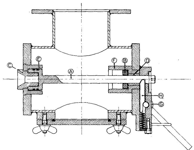
Fig. 4—The operation of the Burchard drain valve
