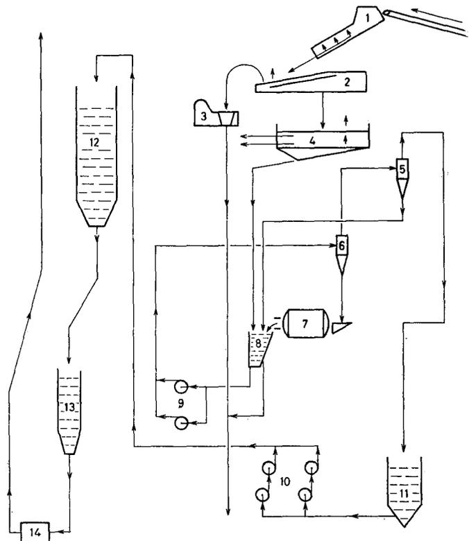
Fig. 2—The washing and screening plant 1. Main feed conveyor. 2. Vibrating bar griddle. 3. Jaw crusher. 4. Double-deck vibrating screen. 5. Secondary cyclone. 6. Primary cyclone. 7. Ball mill. 8. Ball-mill tank and screen. 9. Ball-mill pumps. 10. Storage pumps. 11. Storage tank. 12. Storage silo. 13. Break-pressure tank. 14. Mars pumps.
