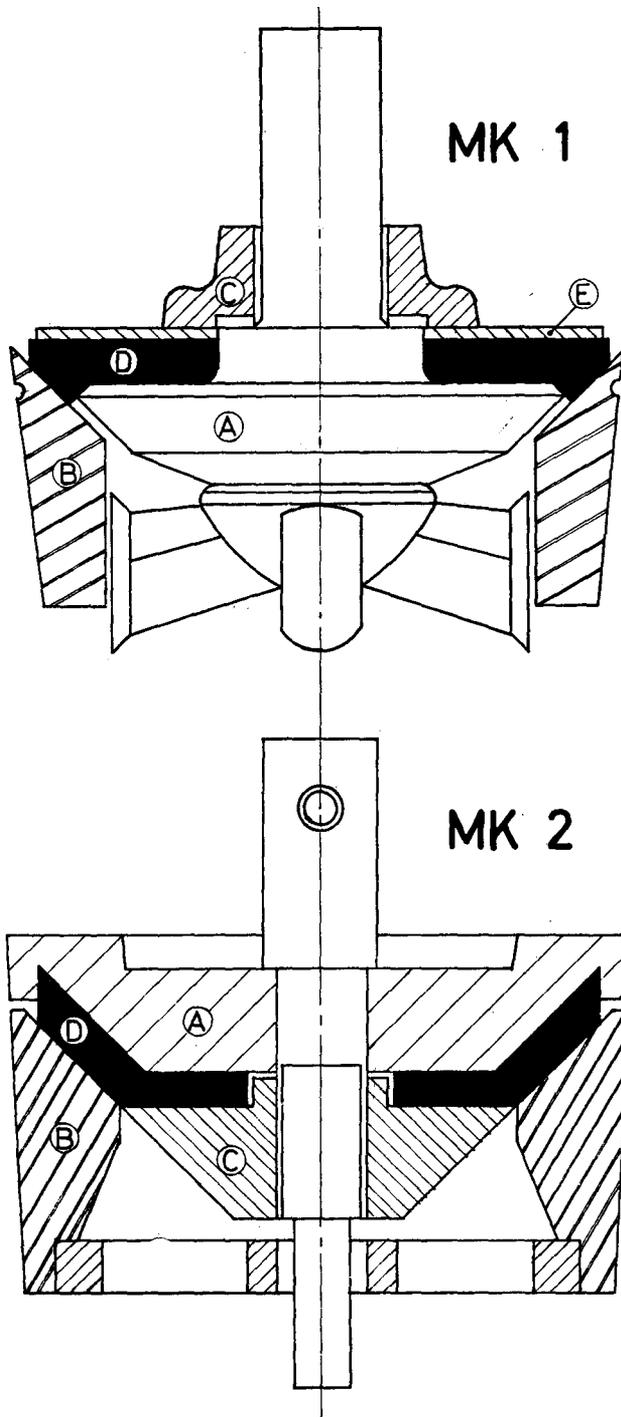
Fig. 3—The original valve, the MK 1, and the valve developed at Vaal Reefs, the MK 2
