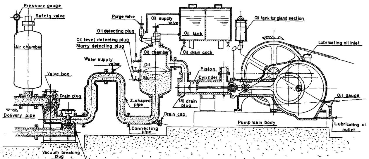
Fig. 5—New layout to eliminate blockages
