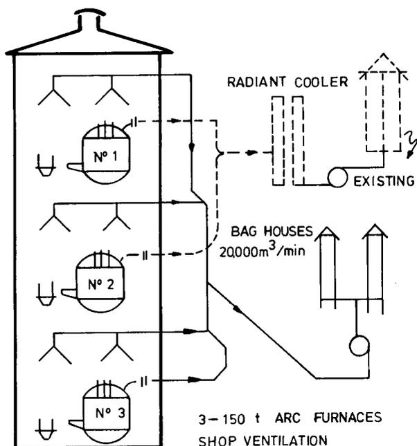
Fig. 13—The fume control system at Iscor's Vanderbijlpark Works
