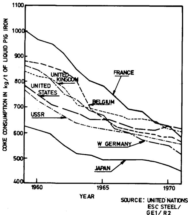
Fig. 2—Consumption of coke by blast furnaces in the principal steelmaking countries, 1960-1971
