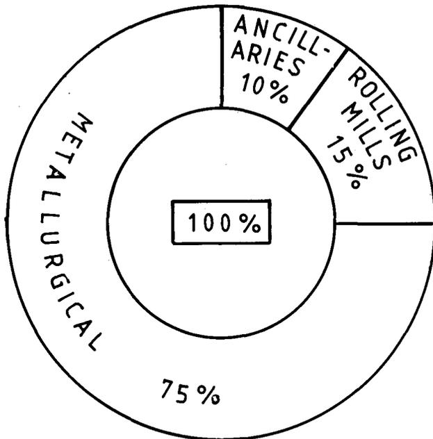
Fig. 5—Contributions to air pollution by the sections of an integrated steelworks
