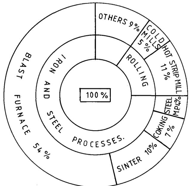
Fig. 3—Energy required for steelmaking
