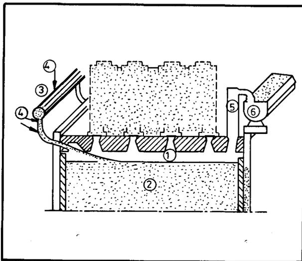
Fig. 8—A preheated-coal charging system
