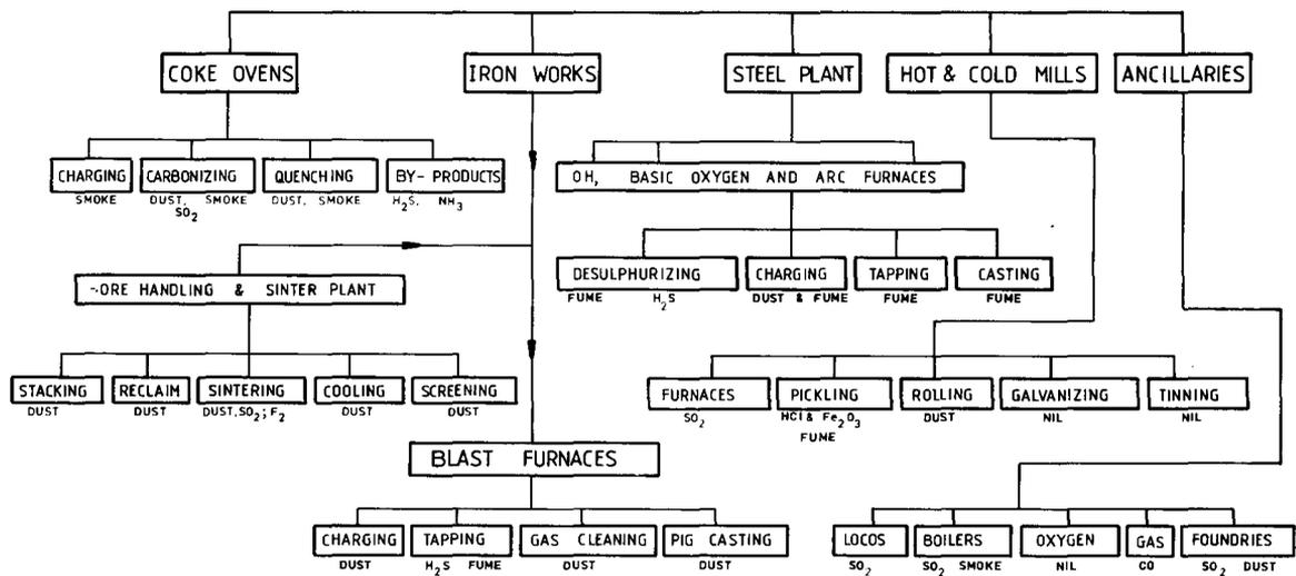
Fig. 4—Possible sources of air pollution in an integrated steelworks
