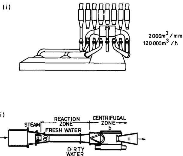
Fig. 10—The extraction and quenching system known as Der Weisse Riese (the White Giant)
