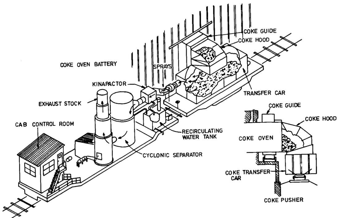
Fig. 9—A completely enclosed pushing system at the Brown's Island coke battery. A hood covers the oven door and the opening of the transfer car during the push, and air-cleaning equipment on the double unit disposes of the trapped emissions
