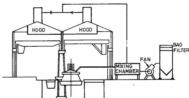
Fig. 14—Combined furnace extraction with full roof extraction
