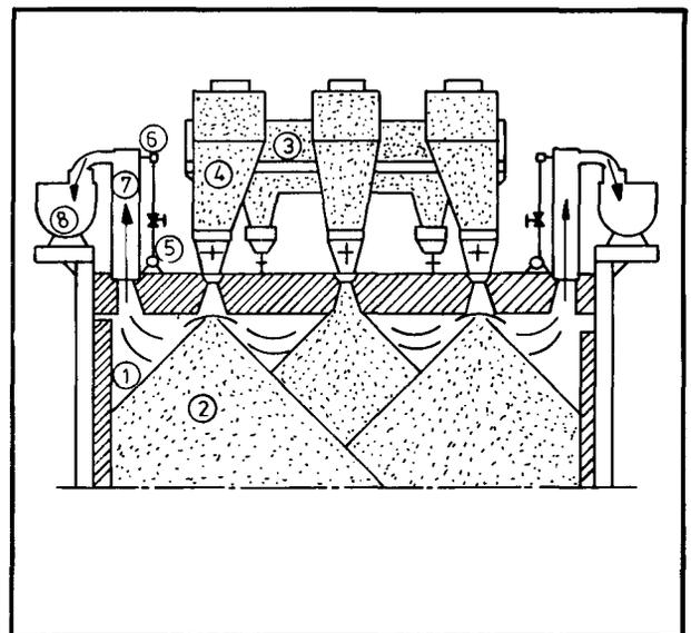
Fig. 6—A gravity charging car with double take-off mains
