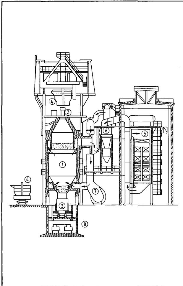
**Fig. 11—Soviet type of dry quenching unit**
