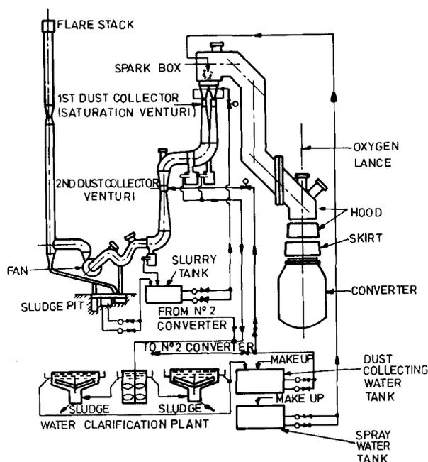
Fig. 12—Simplified diagrammatic arrangement of a spray and dust-collecting water system
