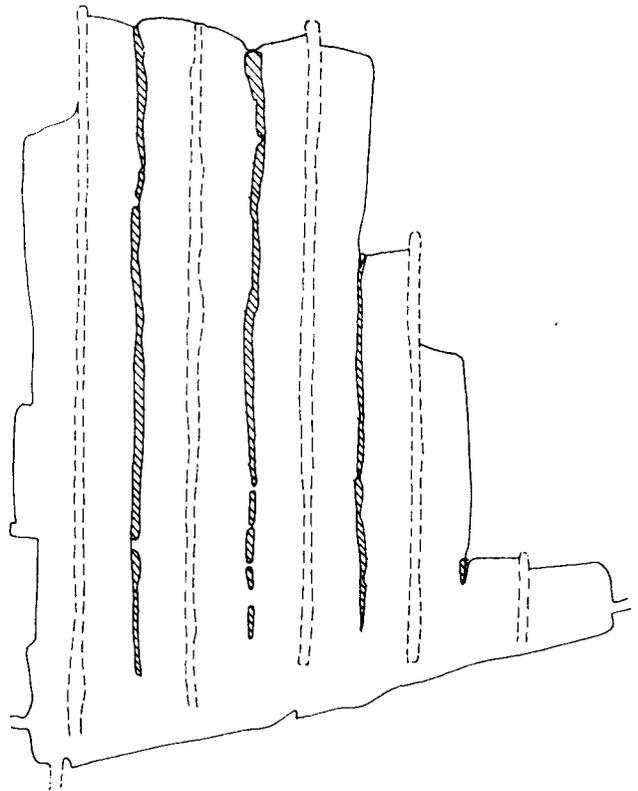
Fig. 5—Layout of crush pillars on the bottom horizon of a reef
