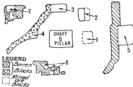
Fig. 2—Block 1 and a portion of Block 2 have been mined, and the stress level at the shaft is critical; 20 per cent extraction
