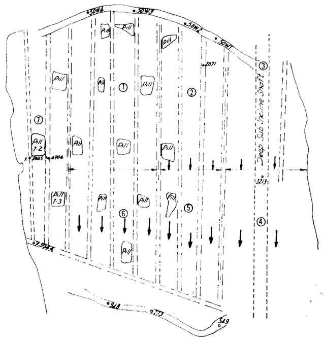
Fig. 6—Layout of a stope supported on pillars, indicating the sequence of pillar extraction and the direction of retreat
