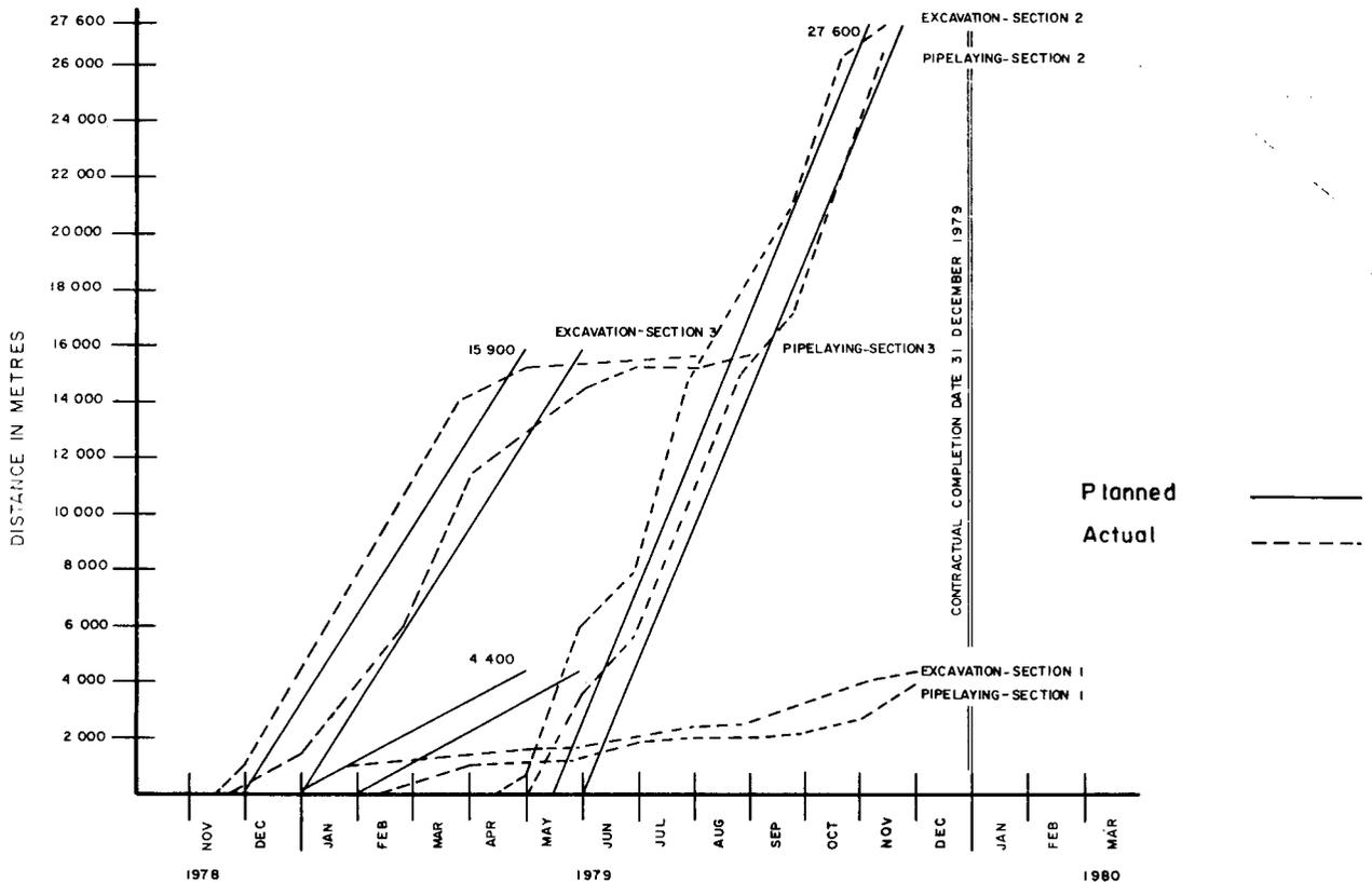
Fig. 4—Graph showing the construction of the main water-supply pipeline at Grootegeluk
