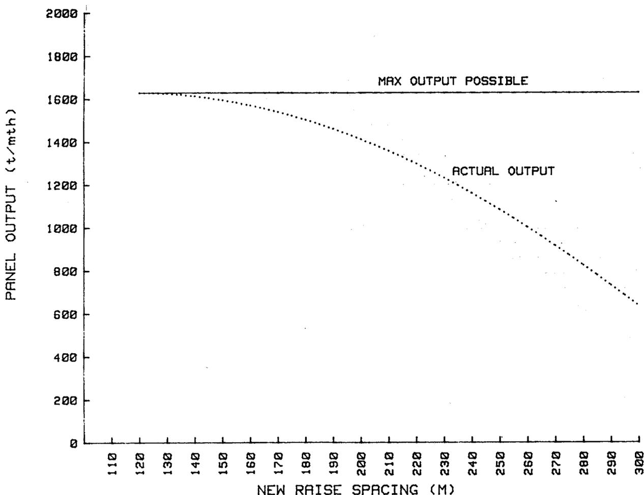
Fig. 1—Average panel output plotted against the new raise spacing
