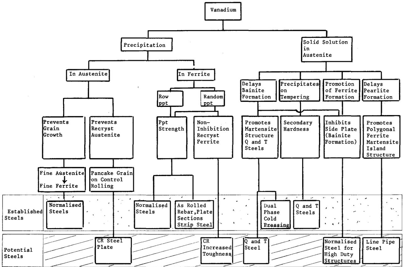
Fig. 1—The metallurgical effects of vanadium in structural steels
