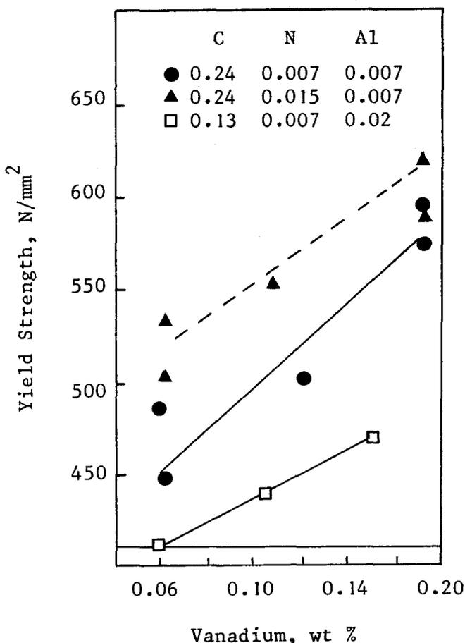
Fig. 3—The effect of vanadium on the yield strength of 30 mm bars (d)
