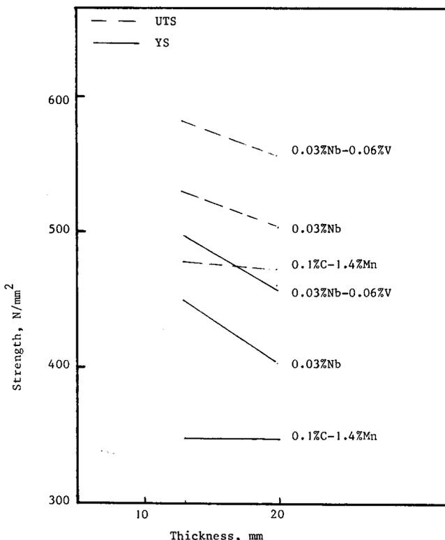
Fig. 4—The effect of thickness on the strength of various steels
