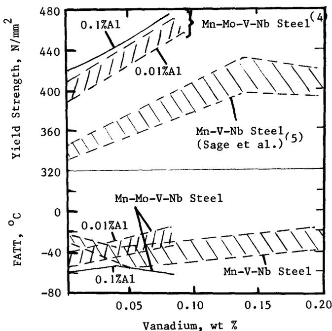
Fig. 5—The effect of vanadium on the yield strength and Charpy V-notch 50% FATT of various steels
