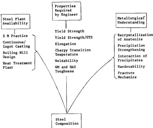
Fig. 2—The parameters controlling the composition of steels
