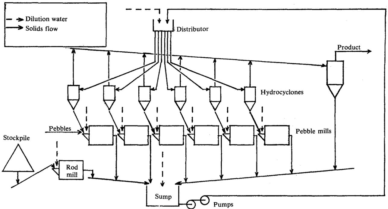
Fig. 1—Flowsheet of the grinding circuit
