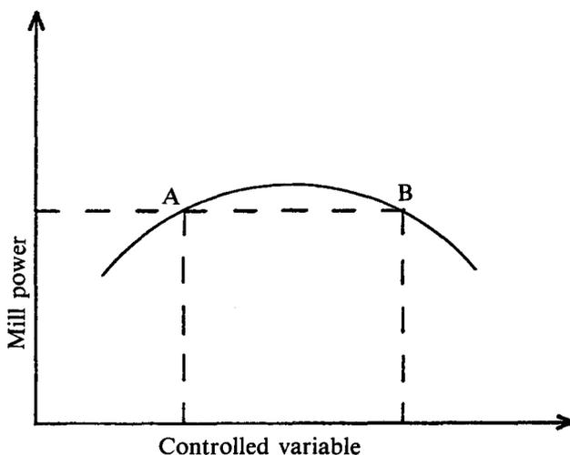
Fig. 6—The absolute value of mill power does not define the state of the controlled variable uniquely
