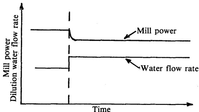
(b) Mill power response at low bulk density
