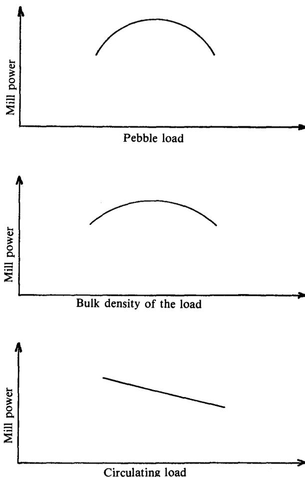
Fig. 3—Relationship of pebble-mill power to the other operating parameters
