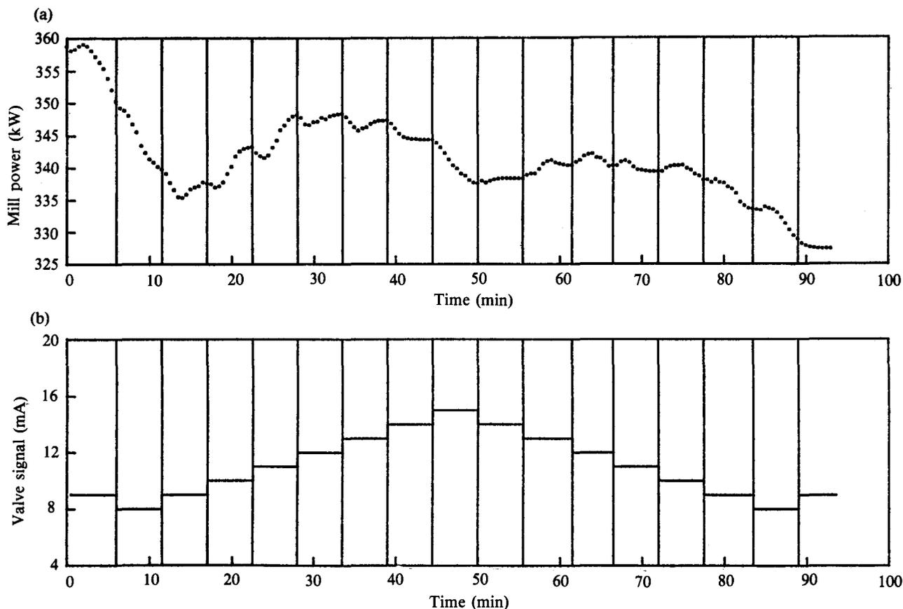
Fig. 4—Response of mill power to changes in the flowrate of dilution water
