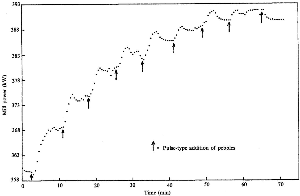
Fig. 7—Mill-power response to the addition of pebbles during the load cycle of the pebble-load controller
