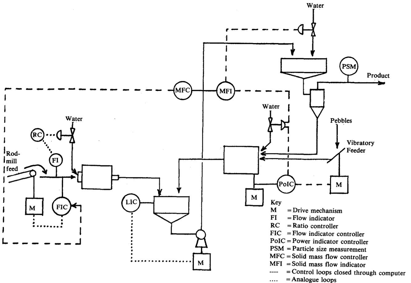
Fig. 2—Schematic diagram of the control loops
