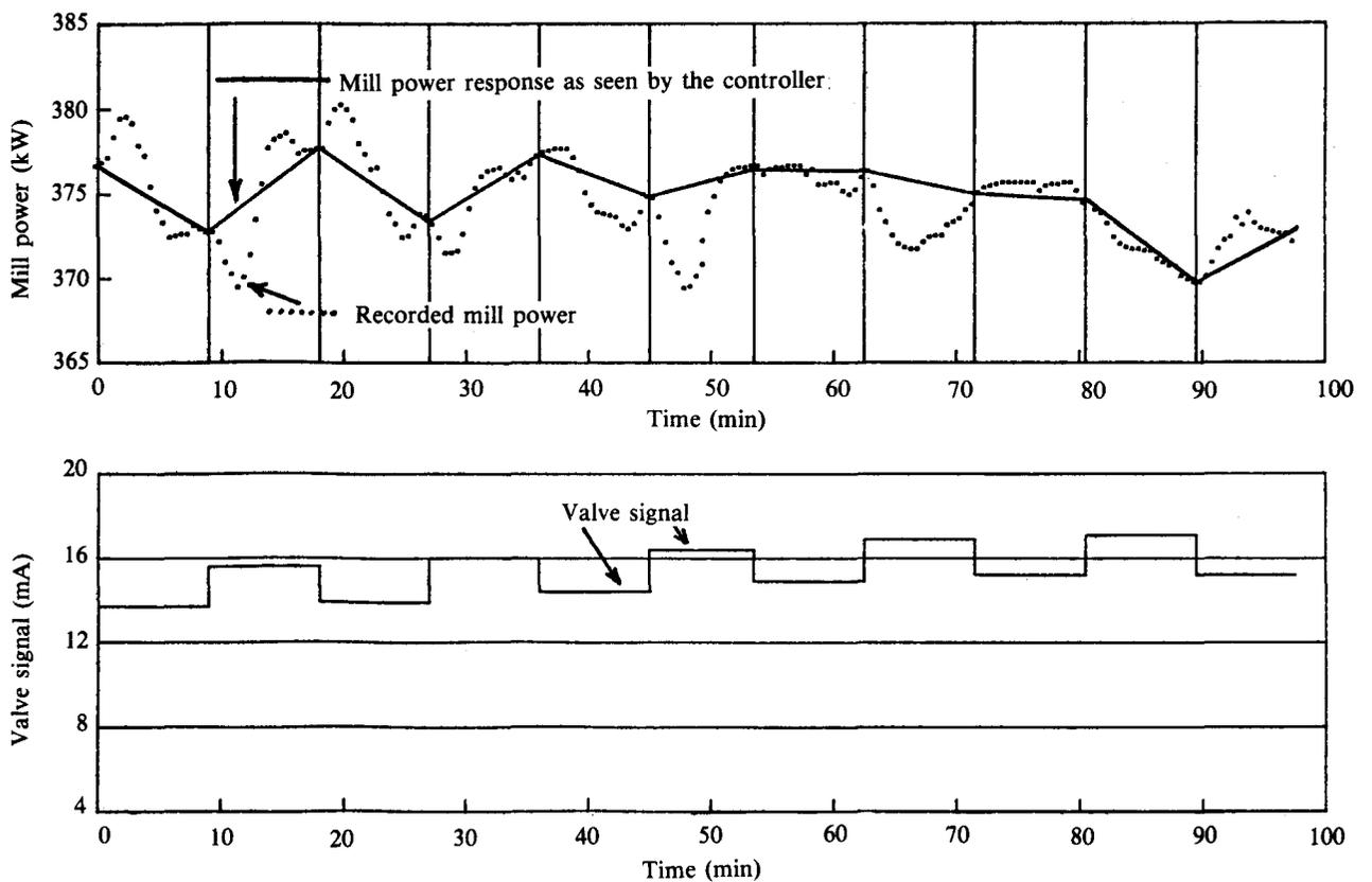
Fig. 8—Operation of the bulk-density controller
