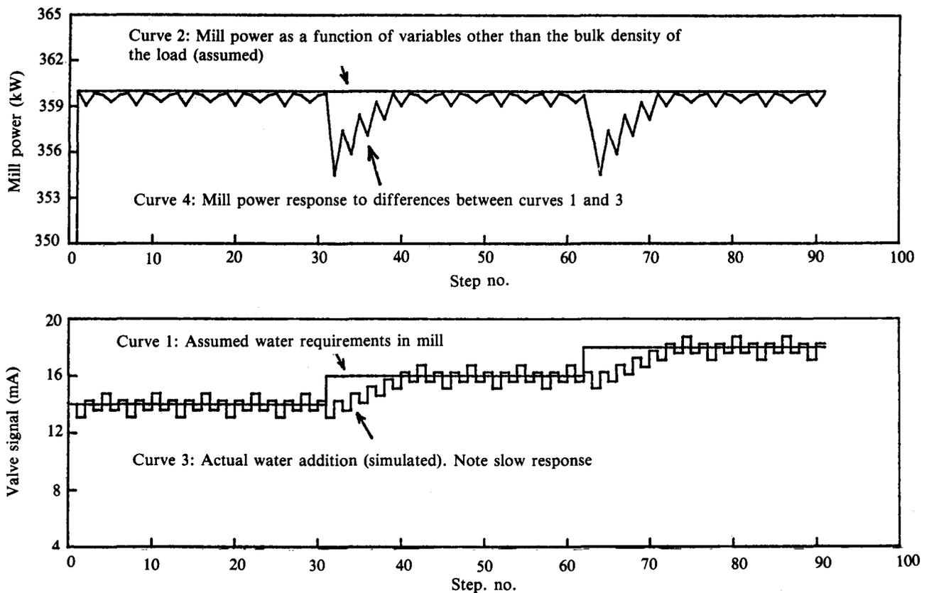
Fig. 9—Slow response of the peak-seeking bulk-density controller
