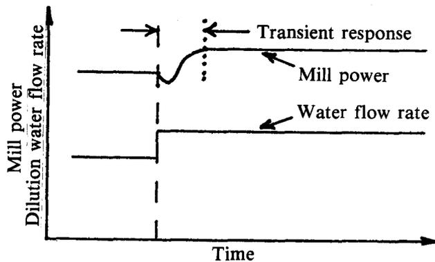
(a) Mill power response at high bulk density
