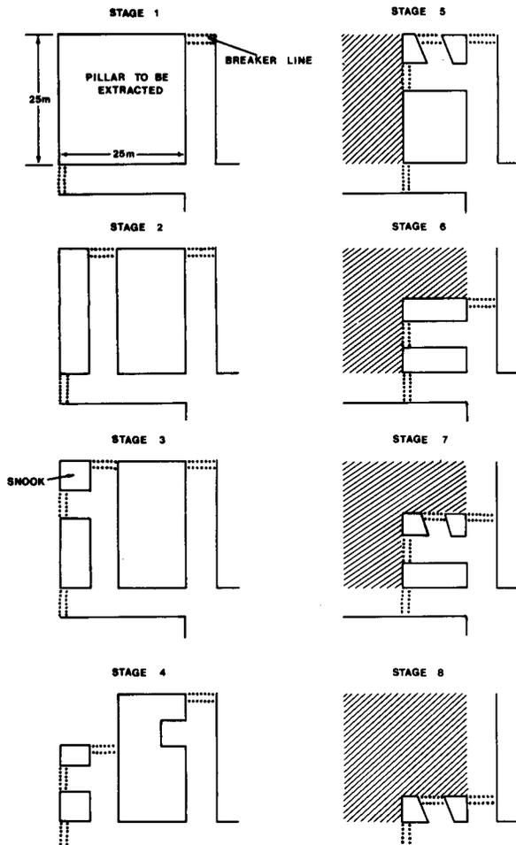
Fig. 5—Sequence of pillar extraction, Method 2
