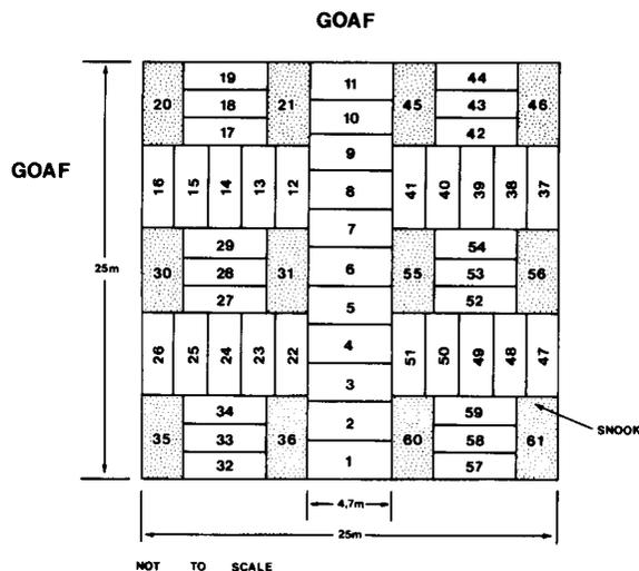
Fig. 4—Sequence of pillar extraction, Method 1
