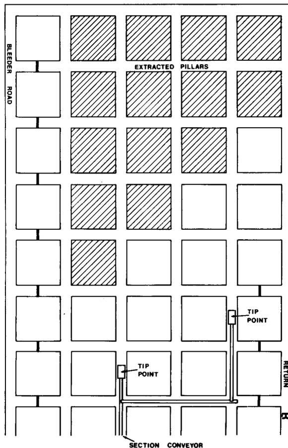
Fig. 3—Panel layout showing inclined stooping line
