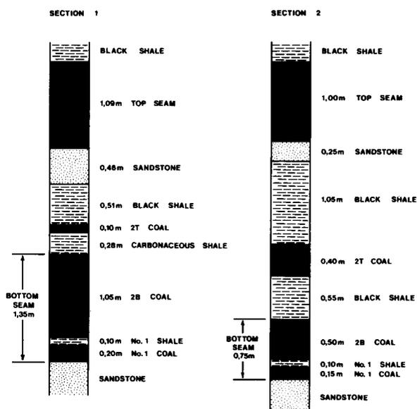
Fig. 1—Typical sections through the coal seams at Durnacol
