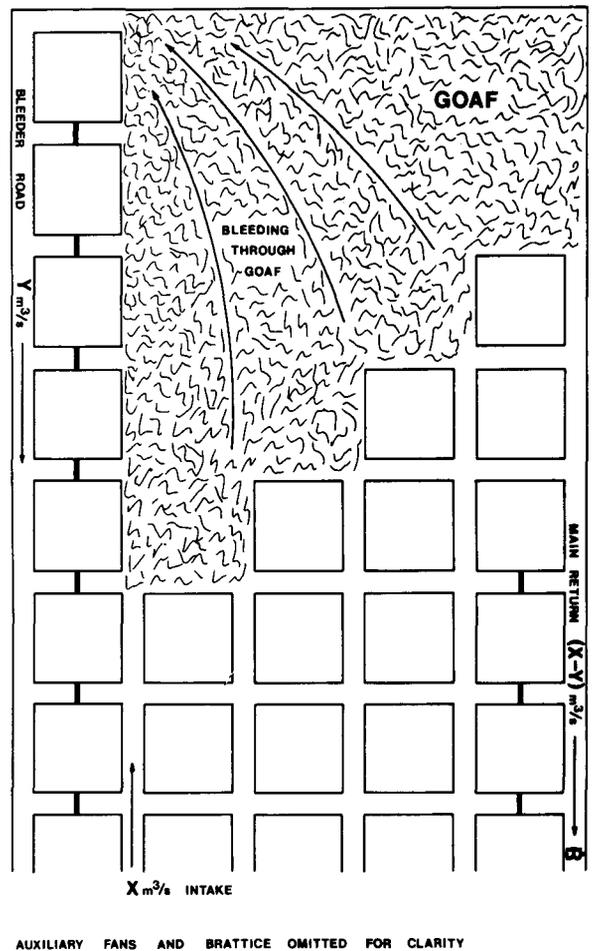
Fig. 6—Typical ventilation arrangement
