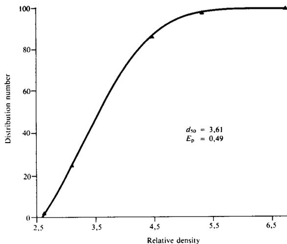
Fig. 5—Adjusted Tromp curve for test A
