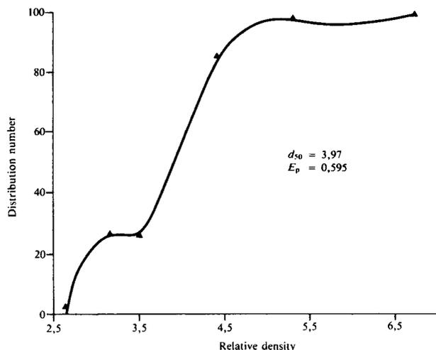
Fig. 4—Tromp curve for reproducibility test A
