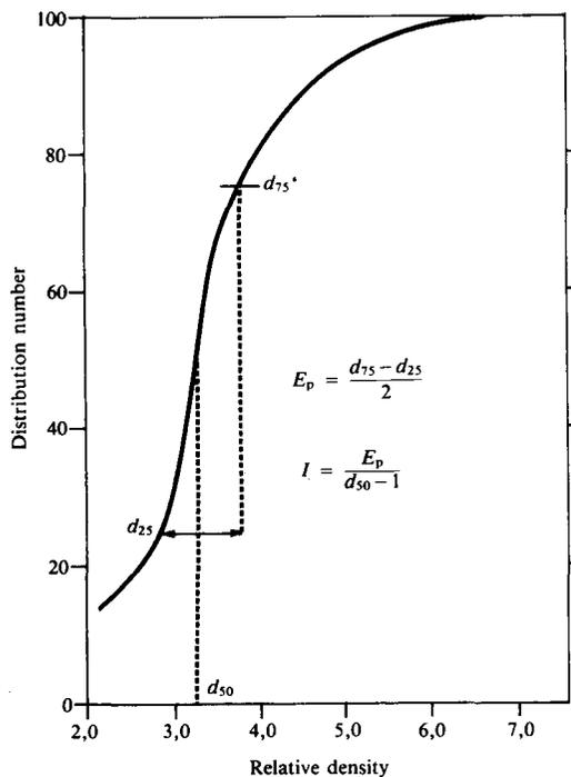
Fig. 1—A Tromp distribution curve
