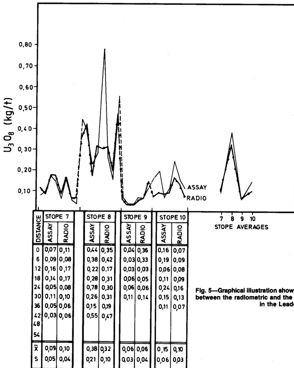
Fig. 5—Graphical illustration showing the close correspondence between the radiometric and the chemical values for uranium in the Leader Reef
