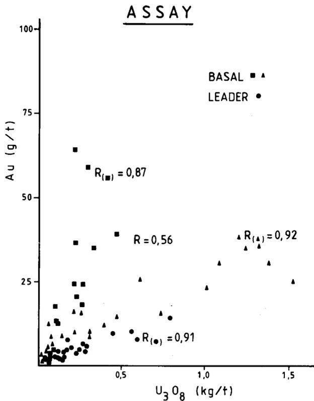
Fig. 7—Linear comparison between the weighted chemical channel averages for gold versus those for uranium. The samples obtained from stopes 1 and 6 on the Basal Reef are depicted by squares
