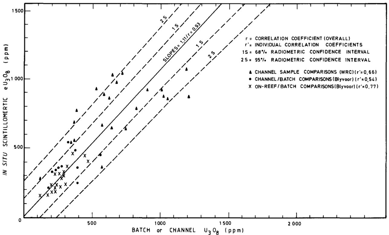
Fig.1—Comparison between *in situ* radiometric  $U_3O_8$  and corresponding batch values or channel-sample assays of  $U_3O_8$  content using a differential face scanner
