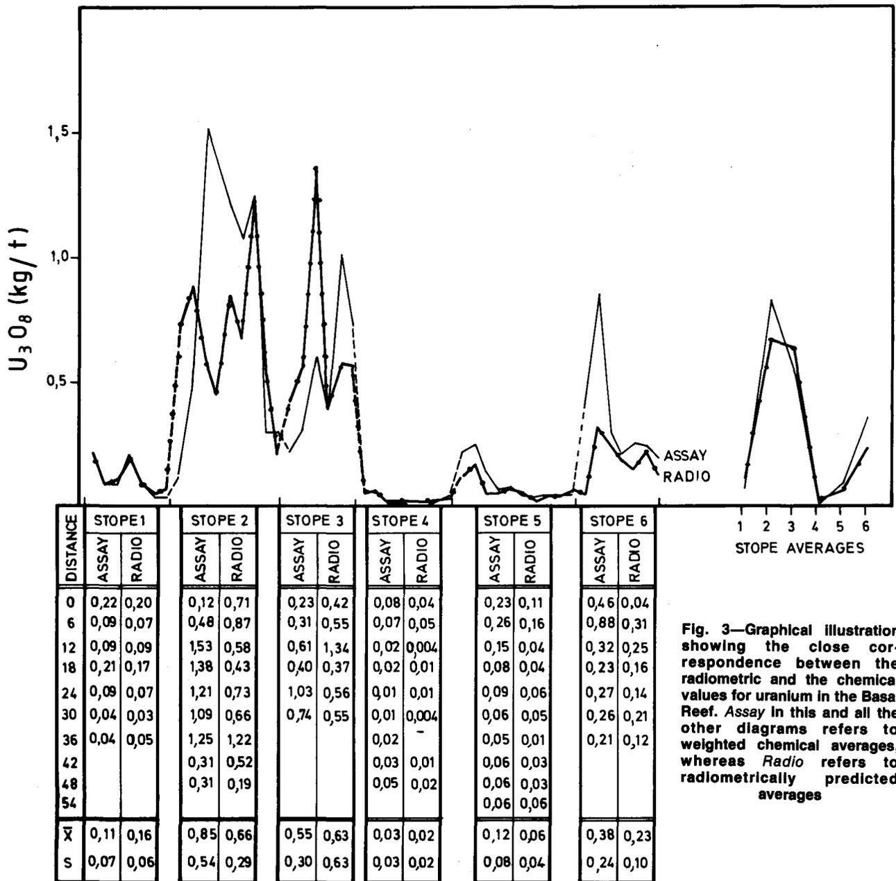
Fig. 3—Graphical illustration showing the close correspondence between the radiometric and the chemical values for uranium in the Basal Reef. Assay in this and all the other diagrams refers to weighted chemical averages, whereas Radio refers to radiometrically predicted averages
