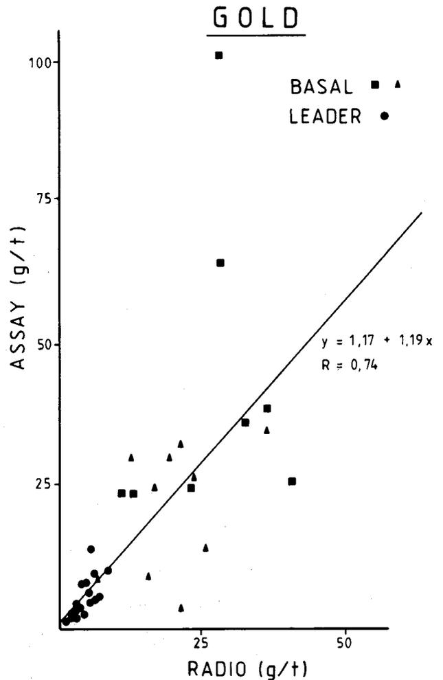
Fig. 9—Linear comparison between the weighted chemical channel averages versus the indirectly predicted radiometric values for gold. The squares represent data obtained from a post-depositional erosion channel on stope 2
