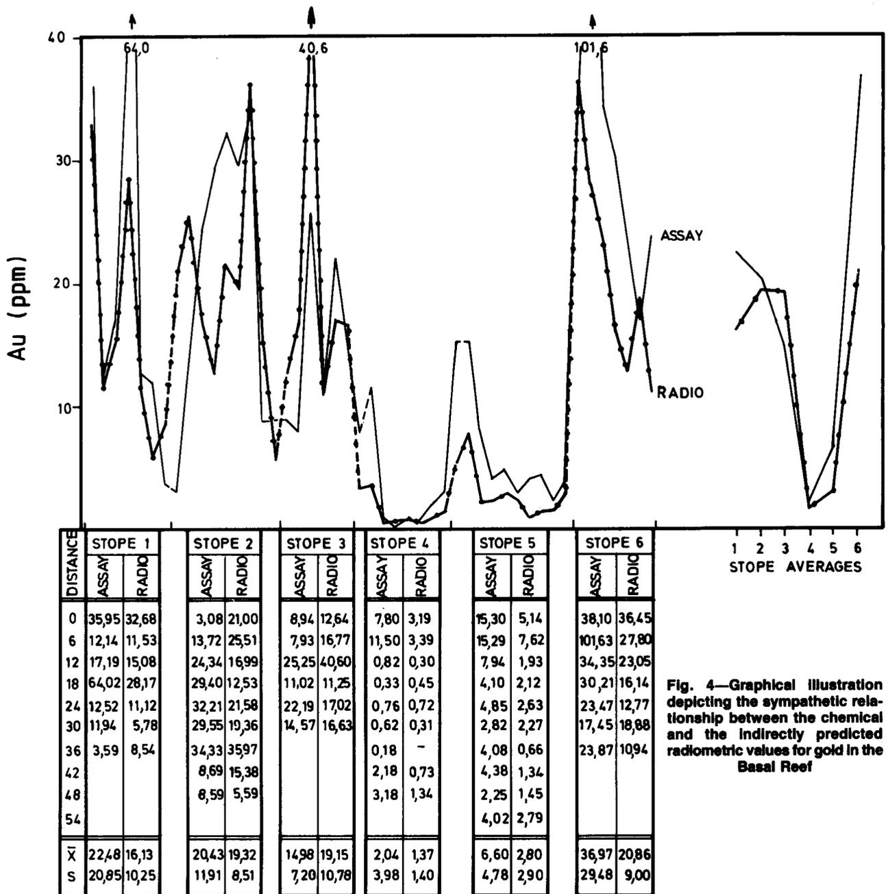
Fig. 4—Graphical illustration depicting the sympathetic relationship between the chemical and the indirectly predicted radiometric values for gold in the Basal Reef
