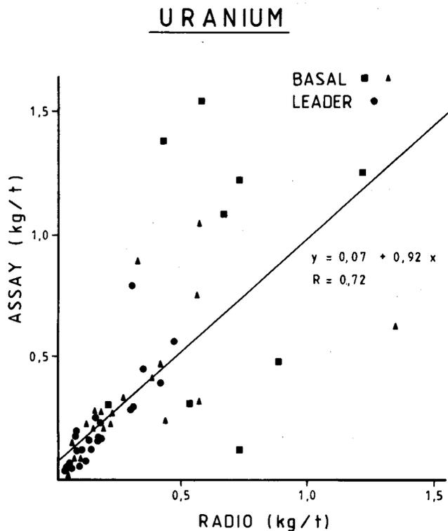
Fig. 8—Linear comparison between the radiometric and the weighted chemical channel averages for uranium. The squares represent data obtained from a post-depositional erosion channel on stope 2
