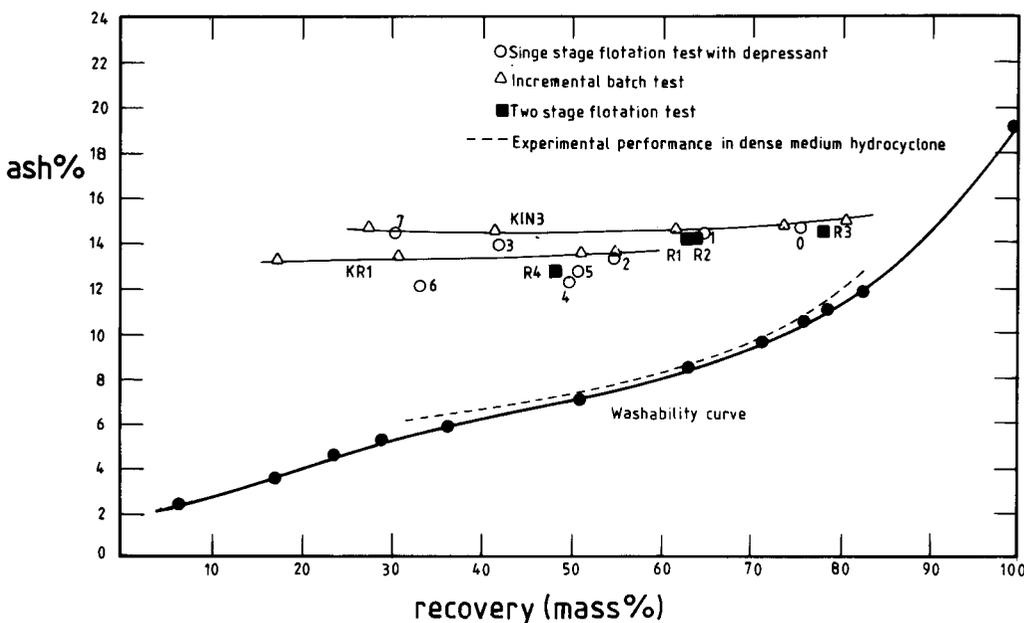
**Fig. 4—Grade-recovery relationship for the batch flotation of Landau fines (the experimental conditions are defined in Tables II and IV)**
