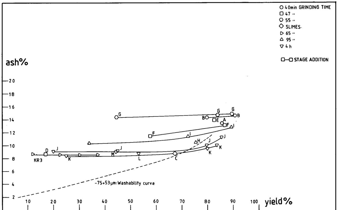
Fig. 9—Grade-recovery relationships in the flotation of reground Landau fines in batch flotation tests
