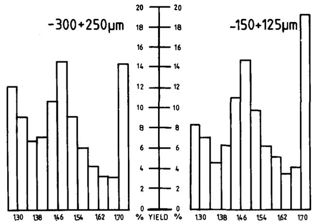
**Fig. 1**—Distribution of density fractions as a function of particle size for Durnacol coal
