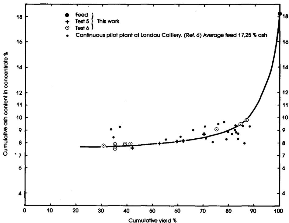
Fig. 11—Grade-recovery relationships in the flotation of ultrafines in the continuous pilot plant. Data obtained on a continuous pilot plant at Landau Colliery are also shown, confirming that the present results are achievable under industrial conditions
