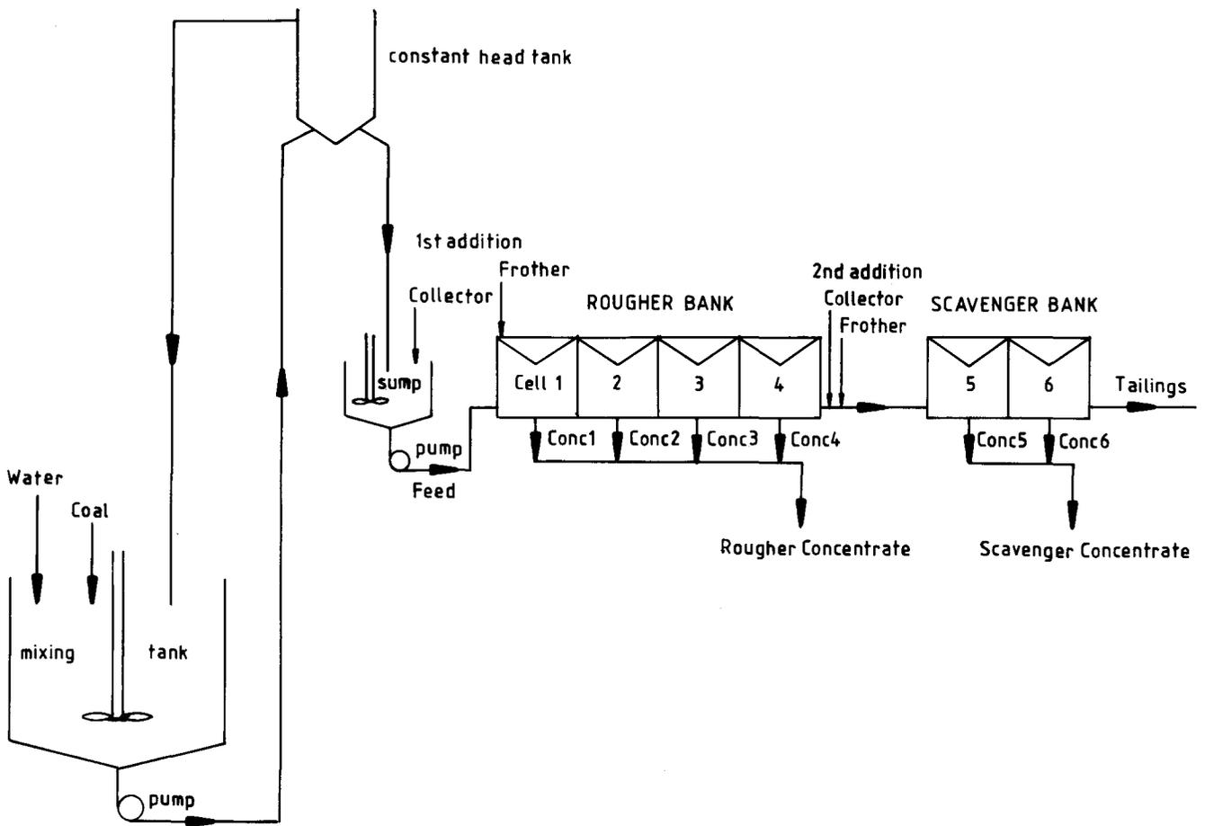
Fig. 10—Layout of the continuous pilot plant for the flotation of ultrafine coal
