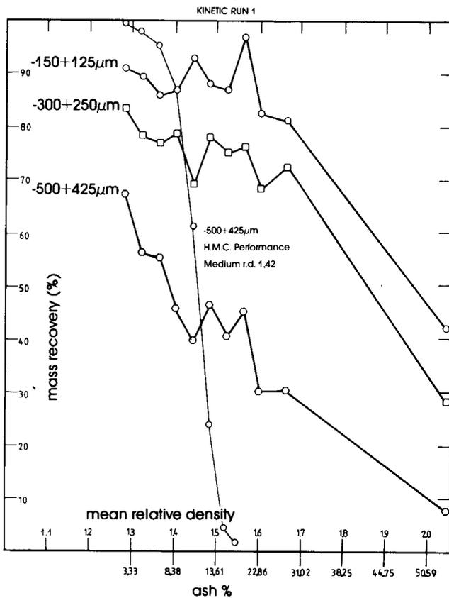
**Fig. 6—Recovery as a function of particle density for 3 particle sizes in a batch flotation test on Landau coal. The measured recoveries for the - 500 + 425  $\mu\text{m}$  fraction of the same coal in a dense-medium cyclone are also shown<sup>1,2</sup>**
