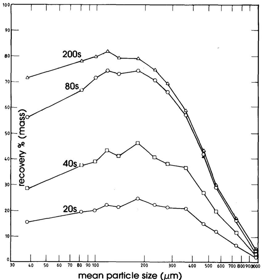
Fig. 5—Recovery as a function of particle size at 4 times in an incremental batch flotation test
