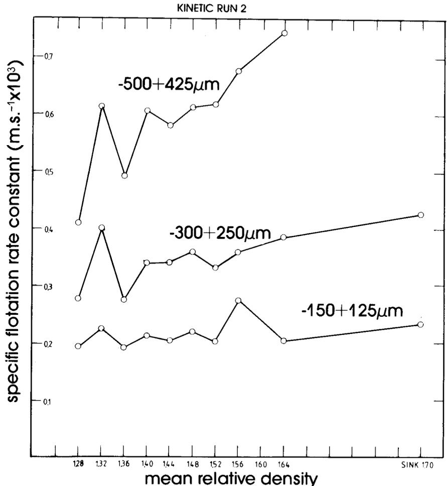
**Fig. 7—Specific flotation rate constant for the floatable component as a function of particle density for 3 sizes**
