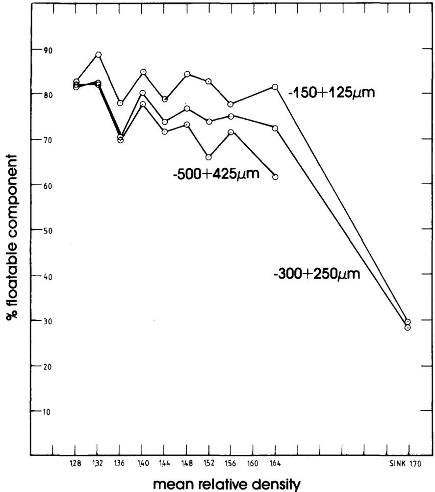
Fig. 8—Percentage of the particles that are floatable as a function of particle density
