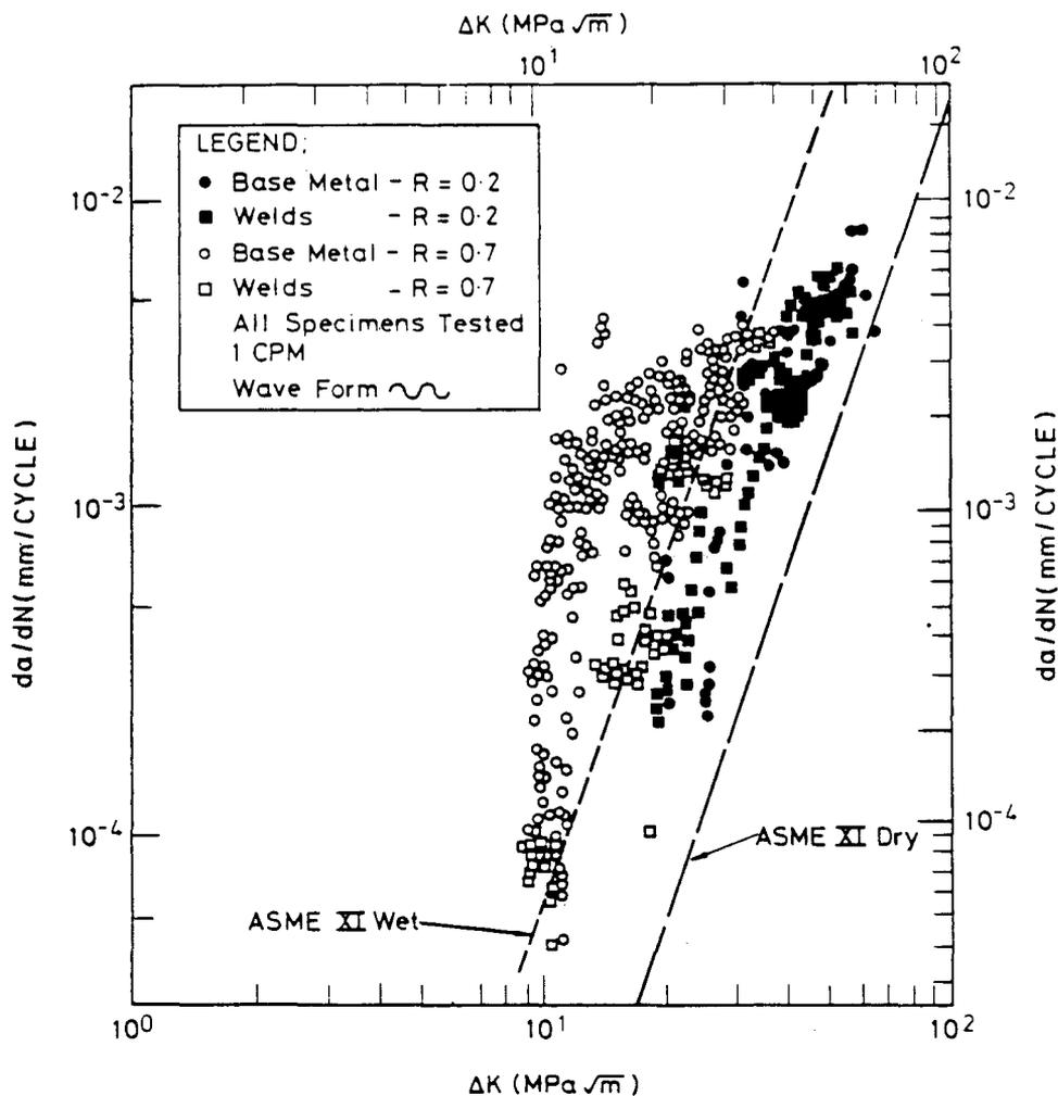
Fig. 3—Corrosion-fatigue data for A533B and A508 base materials and weldments in primary PWR water (after Bamford<sup>4</sup>)
