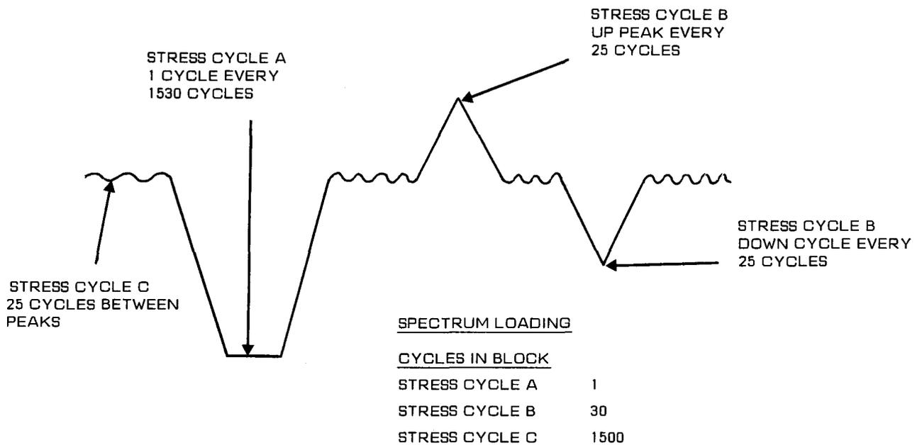
Fig. 14—Conditions of spectrum loading relevant to a working PWR (after Bamford<sup>4</sup>)
