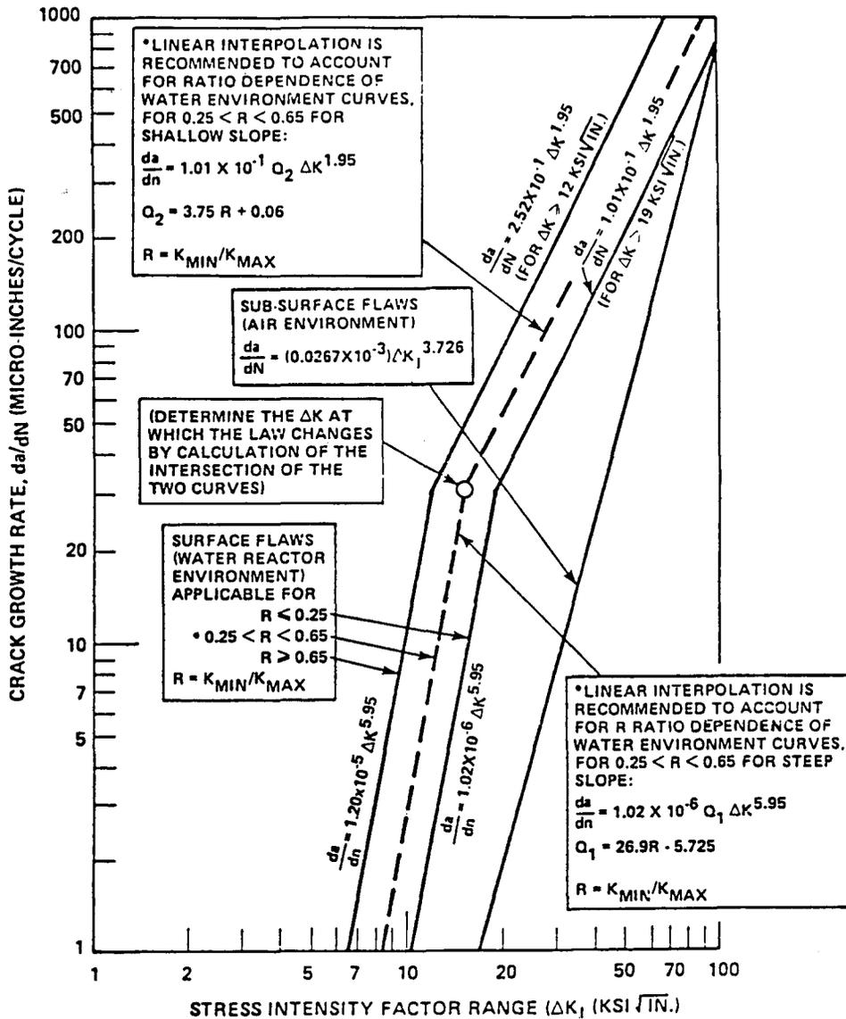
Fig. 4—Reference curves of fatigue-crack growth for carbon and low-alloy ferritic steels, ASME Code, Section XI, 1980 (after Bamford<sup>4</sup>)
