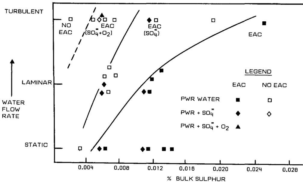
Fig. 7—Susceptibility of RPV steels to EAC (after Atkinson *et al.*<sup>10</sup>)
