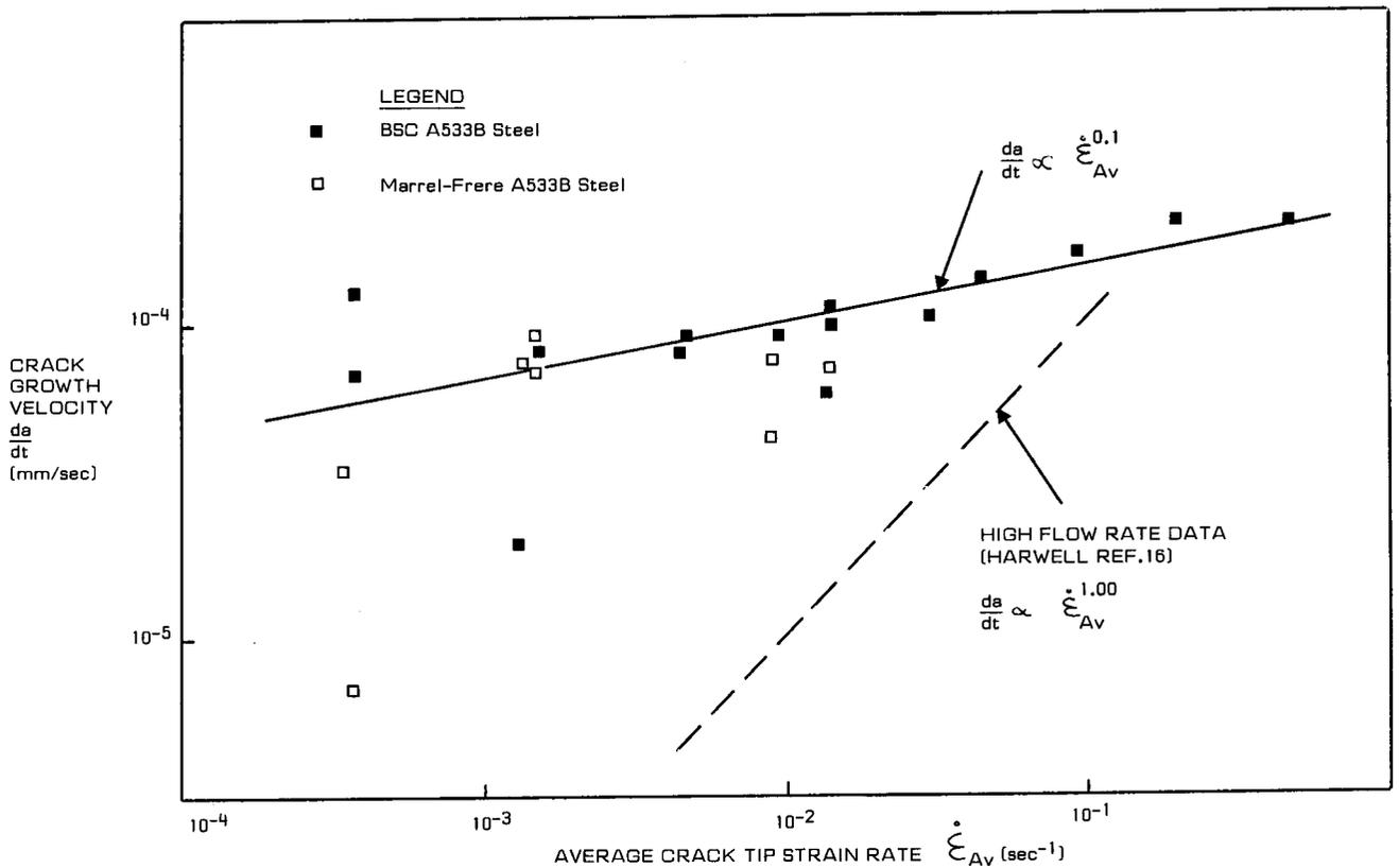
Fig. 8—Velocity of crack growth in A533B steels in PWR water at low and high flowrates as a function of average crack-tip strain rate (after Bulloch<sup>9</sup>)
