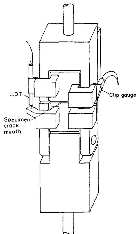
Fig. 2—Crack-monitoring equipment attached to a test specimen
