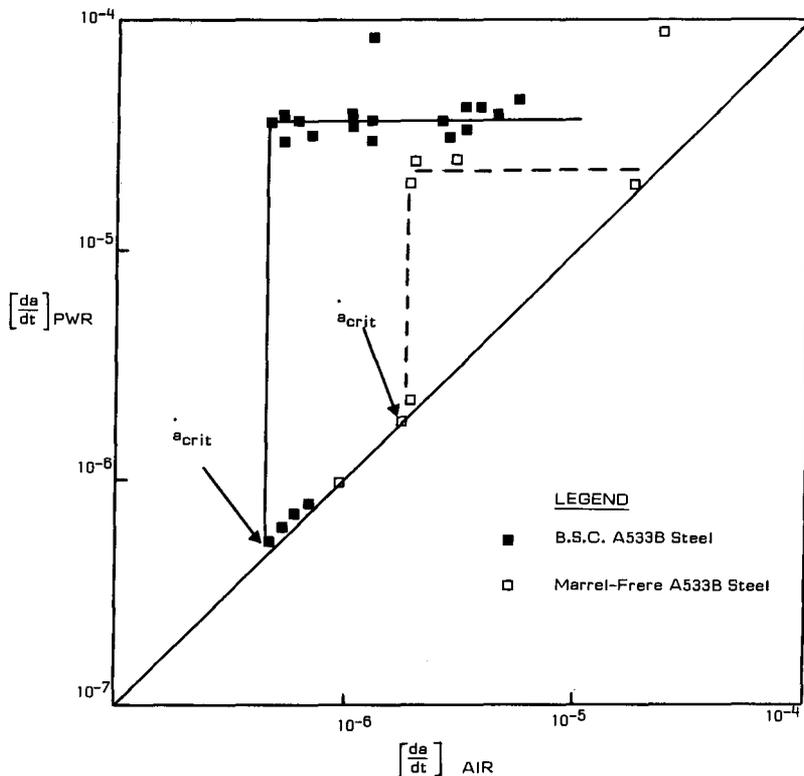
Fig. 10—Velocity of fatigue-crack growth showing the critical crack velocity for two A533B steels (after Atkinson *et al.*<sup>21</sup>).
