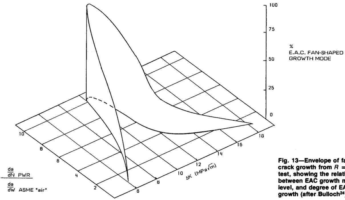
**Fig. 13—Envelope of fatigue-crack growth from  $R = 0,8$  test, showing the relationship between EAC growth mode,  $\Delta K$  level, and degree of EAC growth (after Bulloch<sup>24</sup>)**
