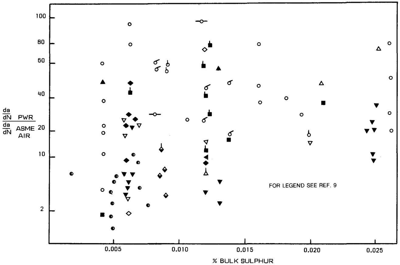
Fig. 6—Literature values of the effect of bulk sulphur on the growth of EAC in RPV materials (after Bulloch<sup>9</sup>)
