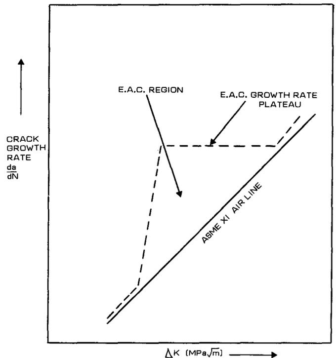
Fig. 11—Growth of EAC associated with the formation of a growth-rate plateau
