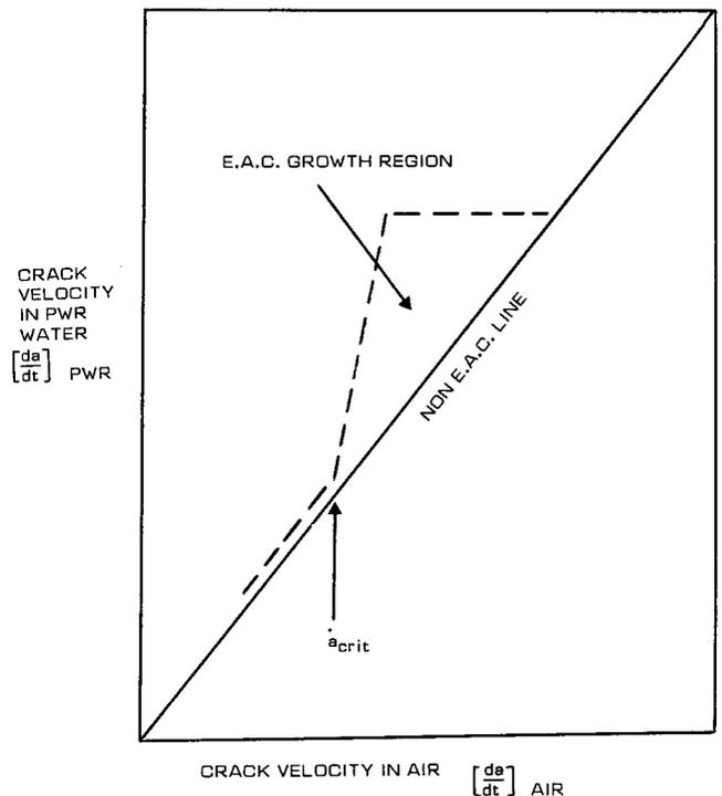
Fig. 9—Crack velocity during the growth of EAC
