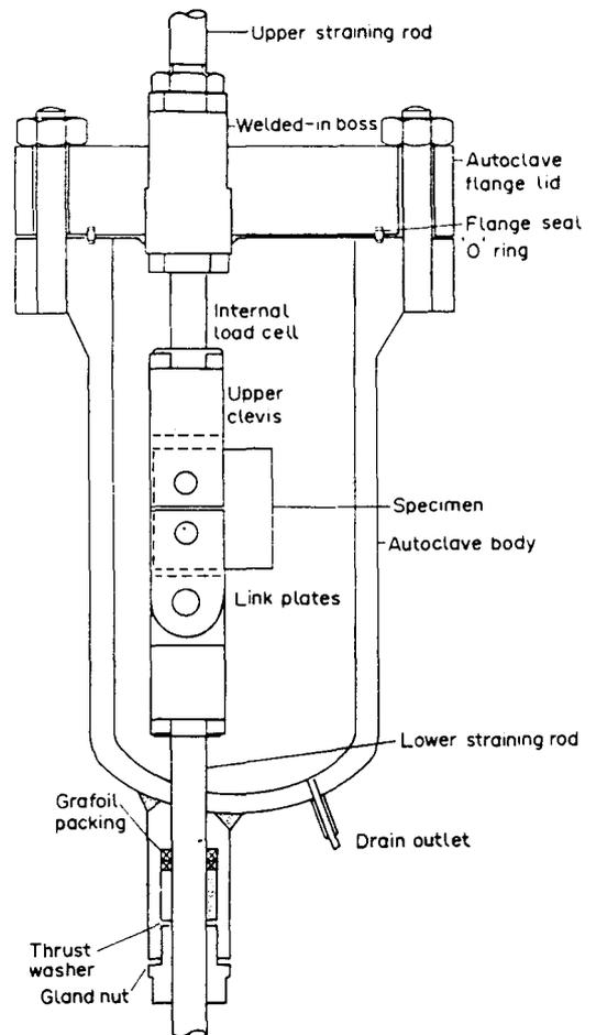
Fig. 1—Section through an autoclave showing the loading arrangement
