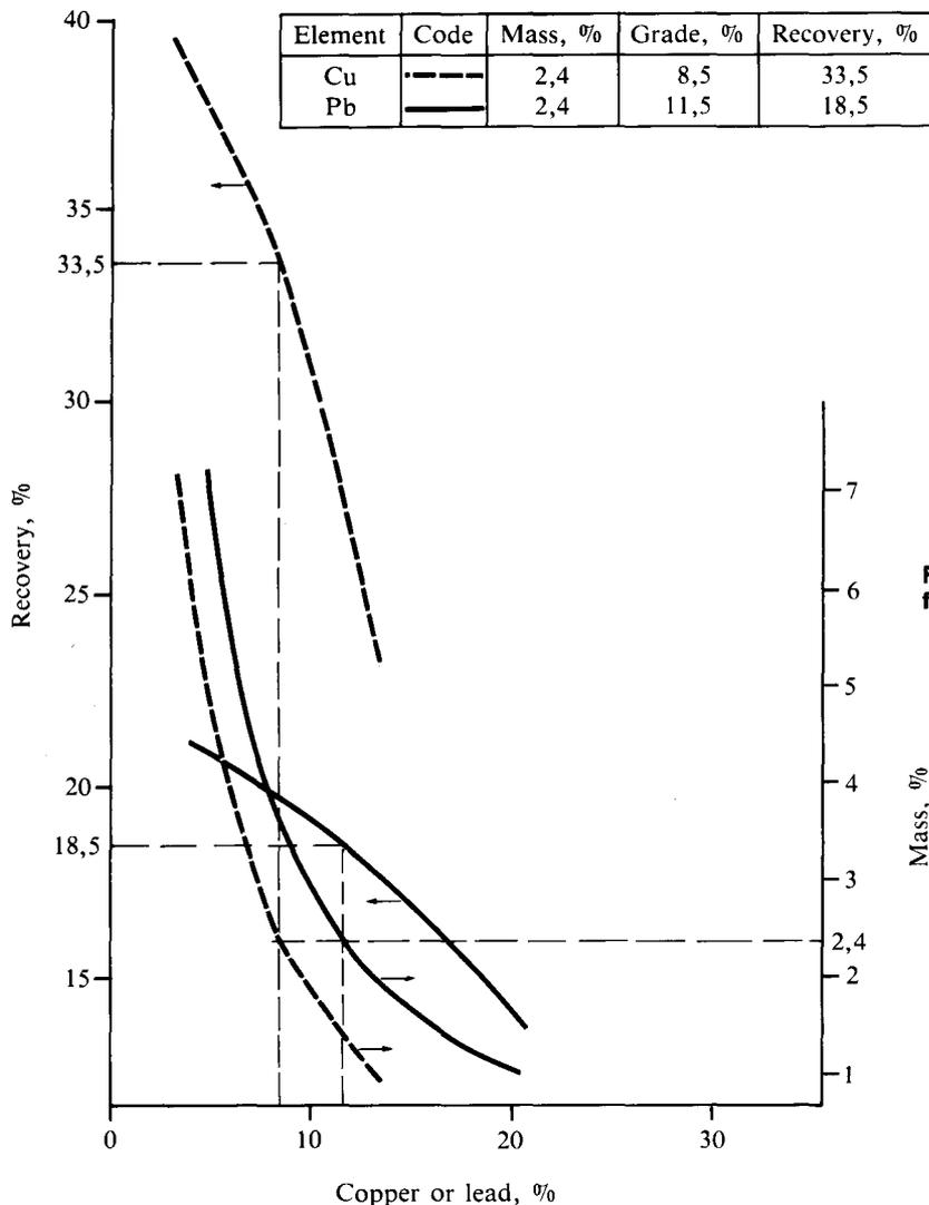
Fig. 7—Results of tabling test on magnetic material from the continuous test on the cyclone underflow from Tsumeb
