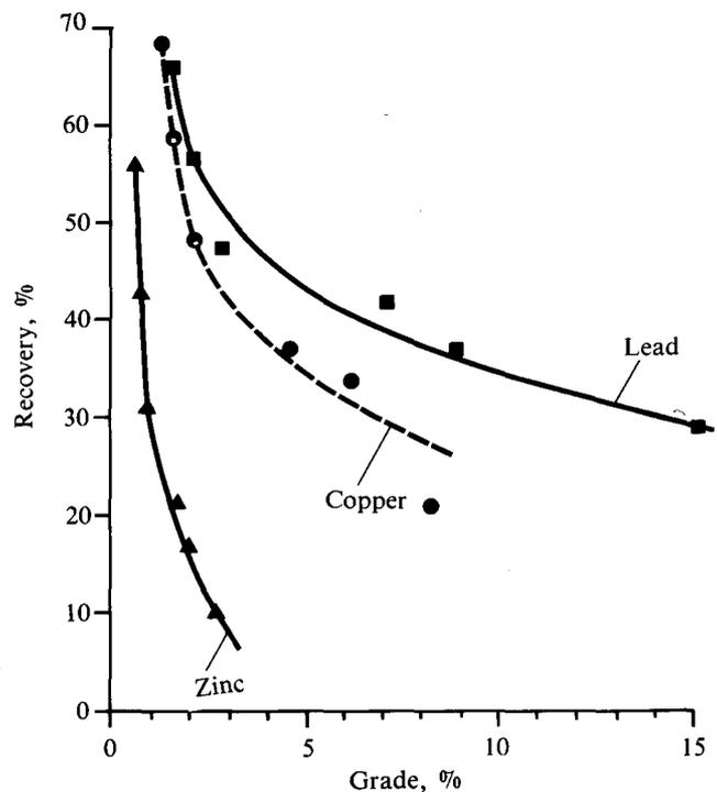
Fig. 3—Spiral tests on deslimed oxide tailings
