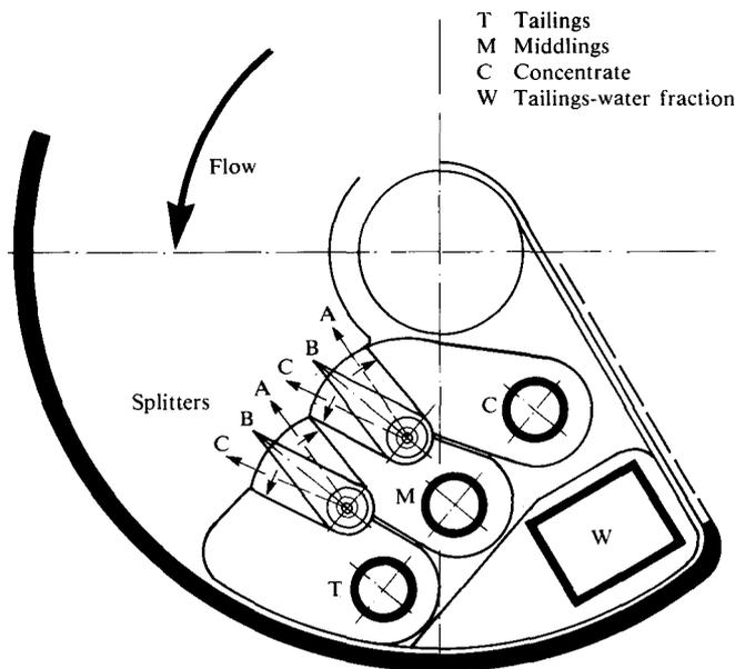
Fig. 1—Position of spiral splitters
