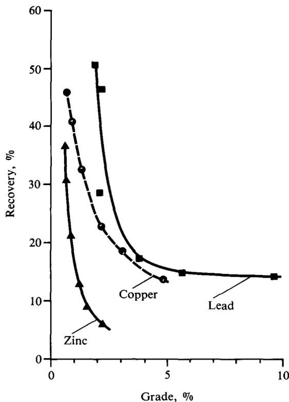
Fig. 2—Spiral tests on oxide tailings
