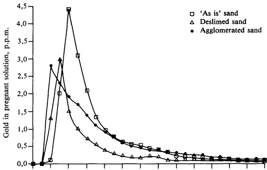
Fig. 7—Operating results from heap leaching in the pilot plant with columns of 225 mm diameter
