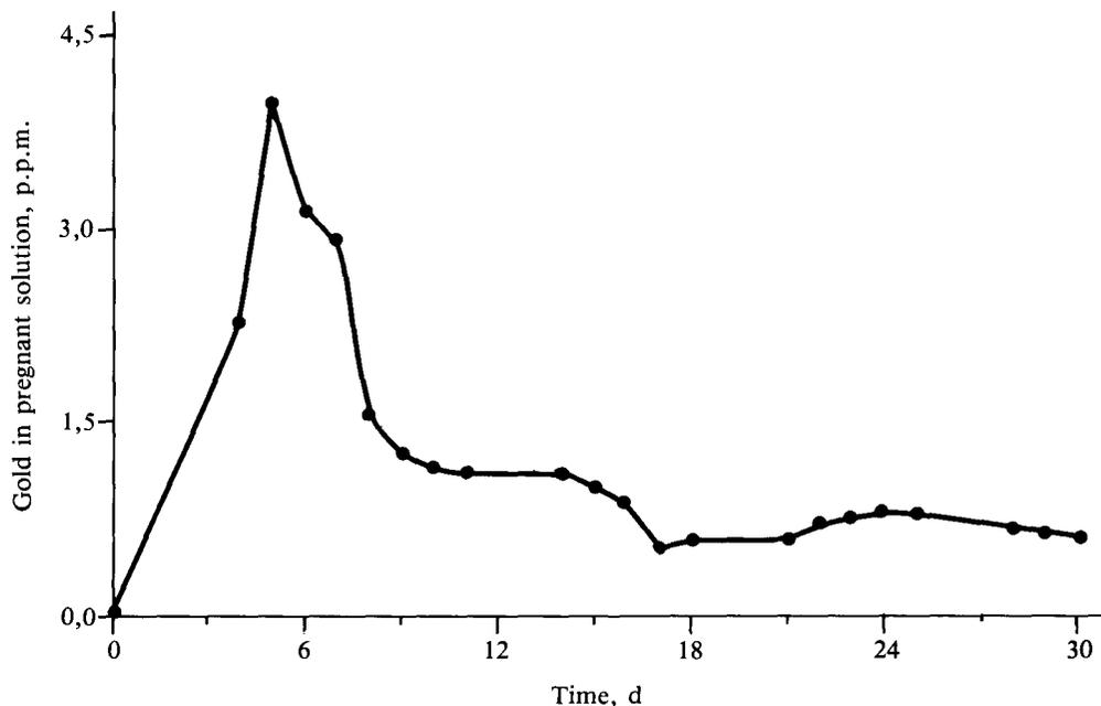
Fig. 3—Examples of operating results from full-scale heap leaching
