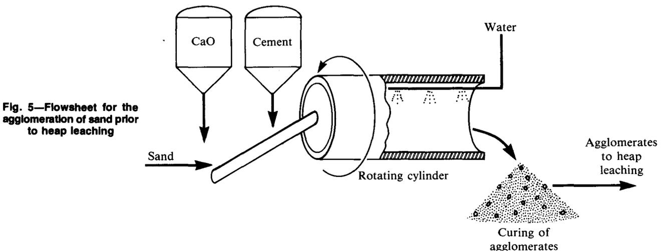
Fig. 5—Flowsheet for the agglomeration of sand prior to heap leaching
