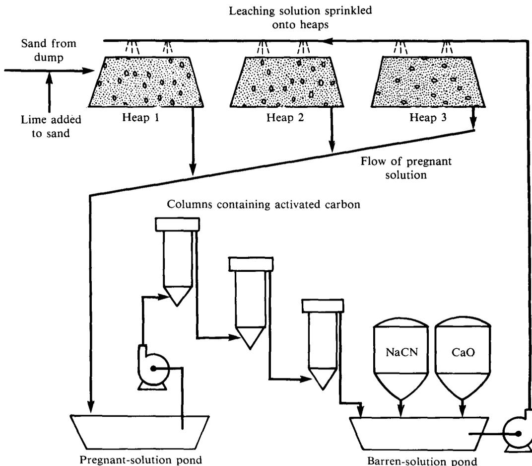
Fig. 2—Flowsheet for the heap-leaching plant at Rand Leases
