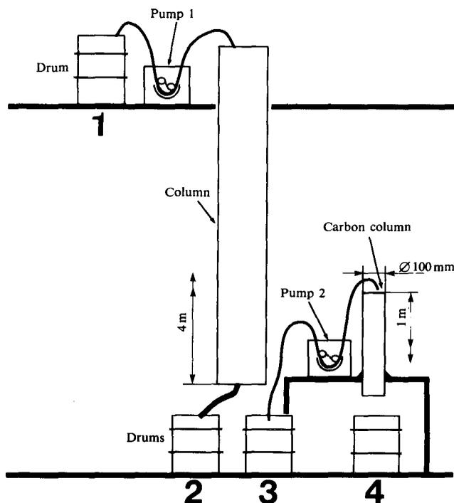
Fig. 6—Layout of the pilot plant for the heap-leaching tests
