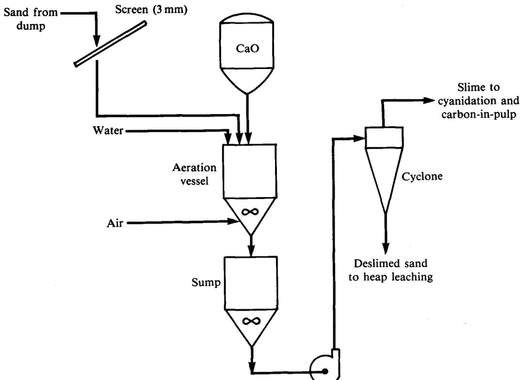
Fig. 4—Postulated flowsheet for the removal of slimes (desliming) from sand
