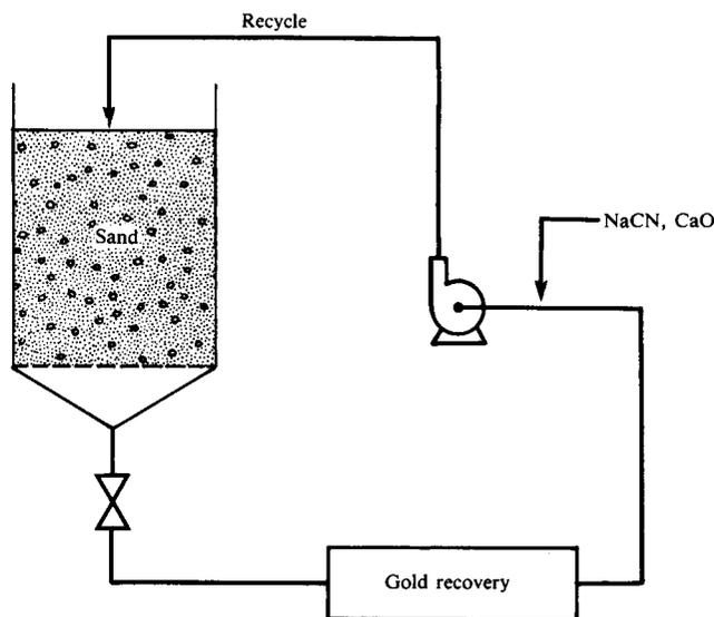
Fig. 1—Schematic representation of vat leaching
